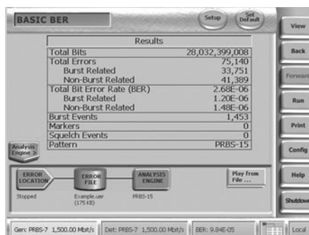
Error Statistics View showing link performance in terms of bit and burst occurrences.
