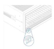
STEP 2: Unsecure the fastening screws and fastening clip
