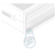
STEP 4: Push module into slot until resistance is felt from the backplane connection
