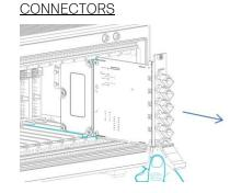
STEP 3: Pull out the module. USE THE FASTENING CLIP TO
