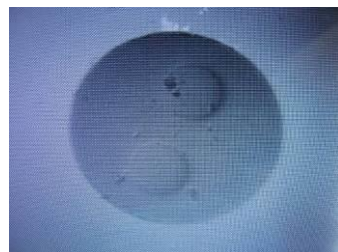
Dirty: Cleaning required
