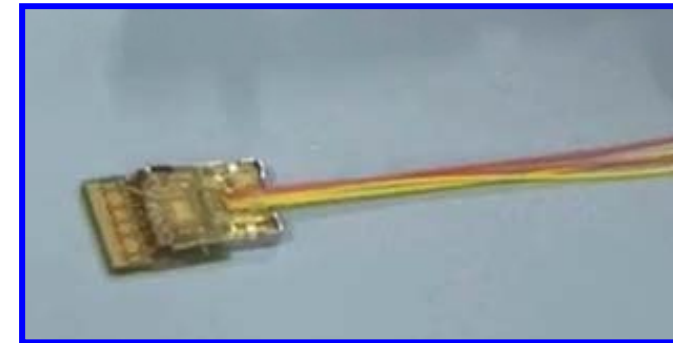
Light Peak Optical Module (12 mm x 11 mm)
