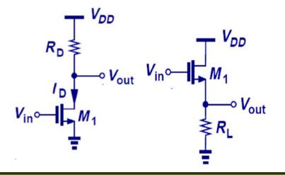
For example, CS and SF can be cascaded for better voltage amplifier performance
