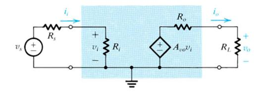
$$v_{o} = \frac{R_{L}}{R_{L} + R_{o}} A_{vo} v_{i} = \frac{R_{L}}{R_{L} + R_{o}} A_{vo} \frac{R_{i}}{R_{i} + R_{s}} v_{s}$$
