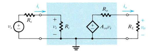
$$v_o = \frac{R_L}{R_L + R_o} A_{vo} v_i = \frac{R_L}{R_L + R_o} A_{vo} \frac{R_i}{R_i + R_s} v_s \sim v_s$$
