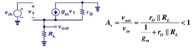
$$A_{v} = \frac{v_{out}}{v_{in}} = \frac{r_{o} \parallel R_{L}}{\frac{1}{g_{m}} + r_{o} \parallel R_{L}} < 1$$
