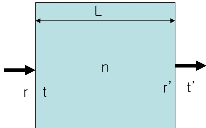
$$T = \frac{I_{out}}{I_{in}} = \frac{(1-R)^2}{(1-R)^2 + 4R \sin^2(kL)} \quad (R = r'^2)$$
