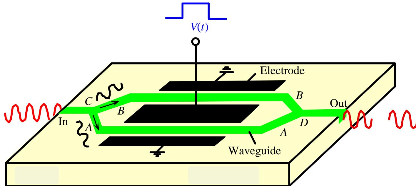
How to modulate Si refractive index with voltage?
