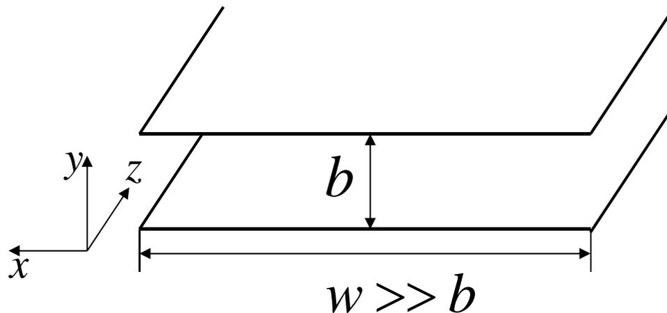
Solve the E&M wave equation  $\nabla^2 \bar{E} - \mu\epsilon \frac{\partial^2 \bar{E}}{\partial t^2} = 0$
