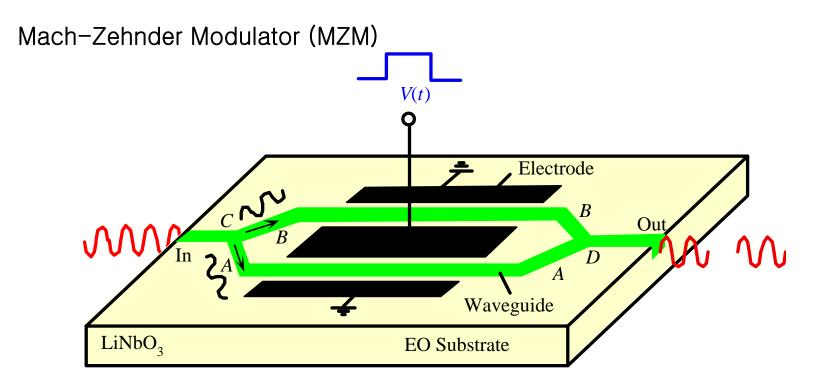
With voltage applied, light travelling in two different arms experiences different amount of phase shift
