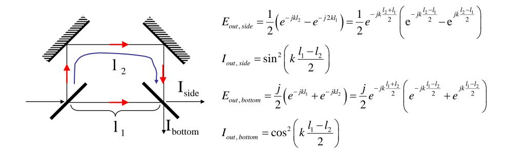
Realize M–Z interferometer with wave devices
