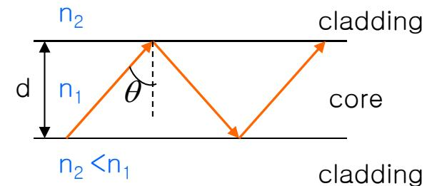
$$e^{-jk_y d} r_{\perp,\parallel} e^{-jk_y d} r_{\perp,\parallel} = 1$$
