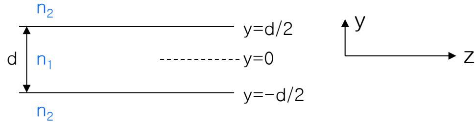
$$\frac{d^2}{dy^2} \bar{E}(y) + (k^2(y) - \beta^2) \bar{E}(y) = 0, \quad k^2(y) = \omega^2 \mu \epsilon(y)$$
