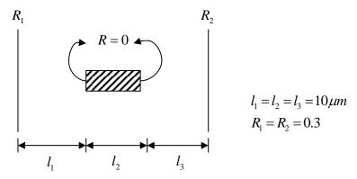
The gain of the material is a function of wavelength and the injected carrier density and is given as  $g(\lambda,n) = a (n-n_0) - b (\lambda - \lambda_0)^2$ , where  $a = 8x10^{-16} \text{ cm}^2$ ,  $n_0 = 1x10^{18}/\text{cm}^3$ ,  $b=4800/\text{cm}-\mu\text{m}^2$ , and  $\lambda_0=1.0\mu\text{m}$ .
