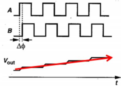
Transfer function for PFD + Charge Pump:
