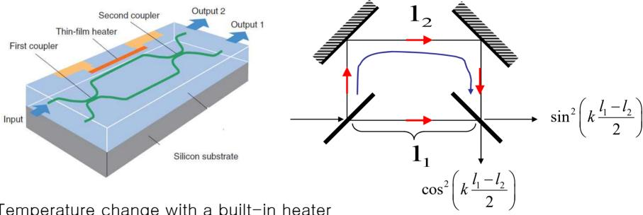
Temperature change with a built-in heater
