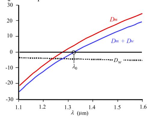
It is possible to control D by changing waveguide structure (Dispersion Flattened Fiber)
