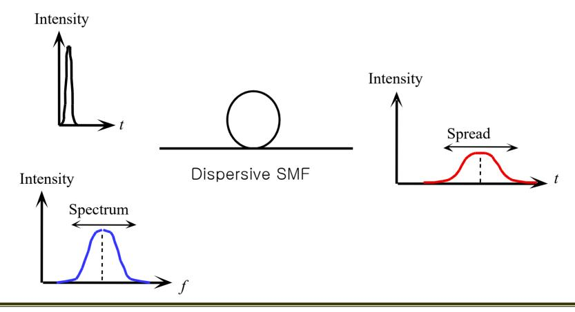
Dispersion exists because  $\beta$  is not not linear with  $\omega$
