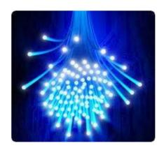
Optical Fiber: Circular dielectric waveguide made up of silica (SiO<sub>2</sub>)
