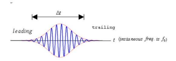
(a)(10) Sketch the frequency-domain spectrum (f>0 only) of the E-field pulse. Clearly indicate important features of your sketch.
