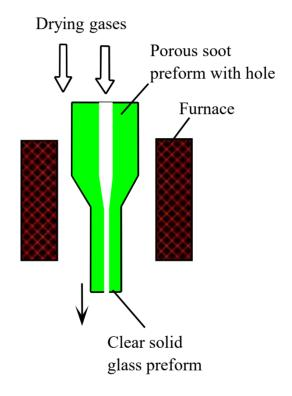
Sintering at 1400-1600 deg C
