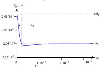
Dispersion in single-mode waveguide: Group velocity depends on frequency
