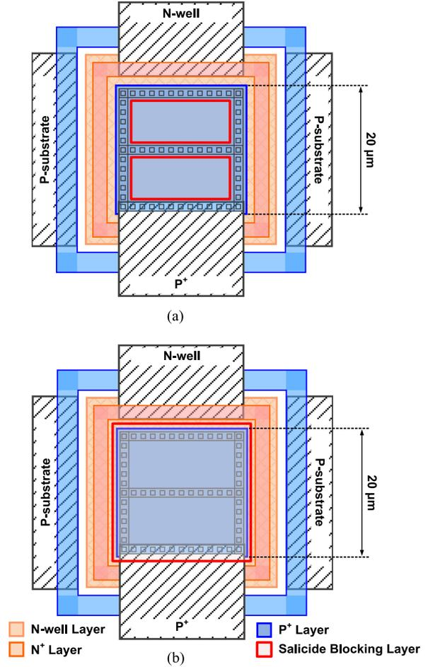
Fig. 16. Simplified  $P^+/N$ -well CMOS-APD layouts (a) with silicide and (b) without silicide [42].
