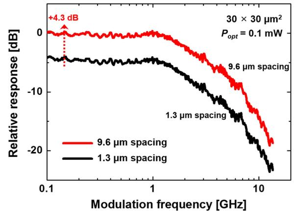
Fig. 19. Measured photodetection frequency responses of CMOS-APDs having (a)  $1.3 \mu\text{m}$  and (b)  $9.6 \mu\text{m}$  spacing multi-finger electrodes on optical windows.
