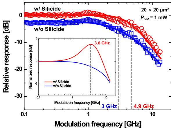
Fig. 17. Measured and simulated photodetection frequency responses of CMOS-APDs with and without silicide. Hollow circles represent measured data and solid lines simulated results with the equivalent circuit model. The inset shows normalized photodetection frequency responses of CMOS-APDs without the photogenerated-carrier transit time [42].
