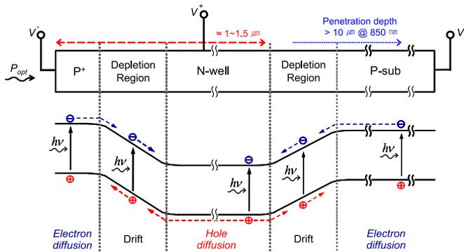
Fig. 7. Simplified band diagrams for  $P^+/N$ -well CMOS-APDs.
