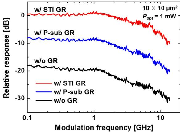
Fig. 12. Measured photodetection frequency responses of the fabricated CMOS-APDs without GR, with P-sub GR, and with STI GR [38].
