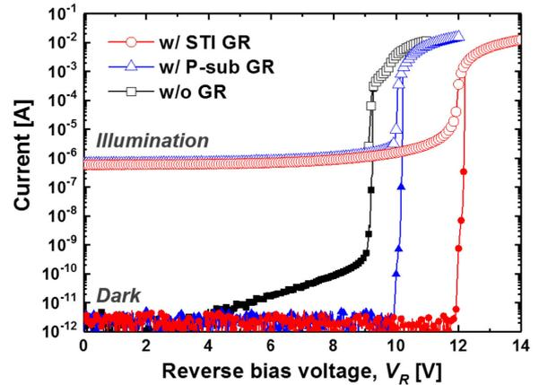
Fig. 11. Current-voltage characteristics of the CMOS-APDs under dark and illumination conditions: (i) w/o GR, (ii) w/ P-sub GR, and (iii) w/ STI GR [38].
