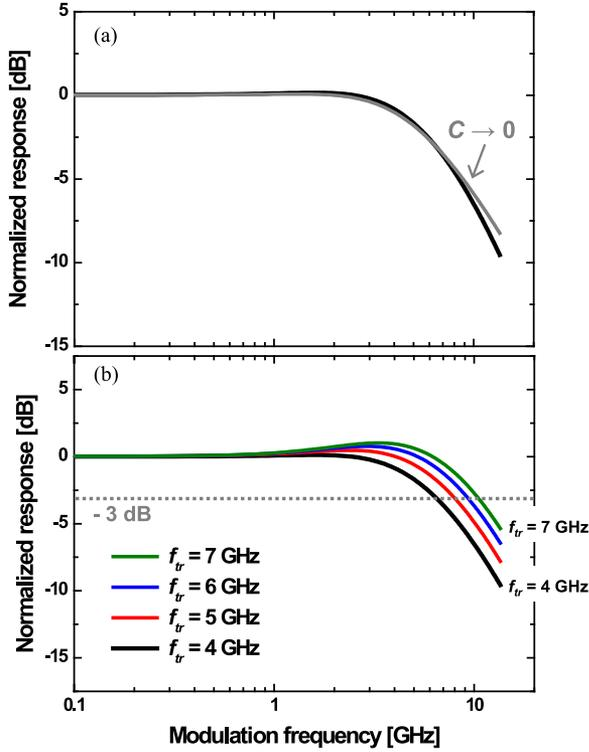
Fig. 15. Normalized photodetection frequency responses of the  $10 \times 10 \mu\text{m}^2$  CMOS-APD (a) with minimization of capacitance and (b) with increasing  $f_{tr}$ .
