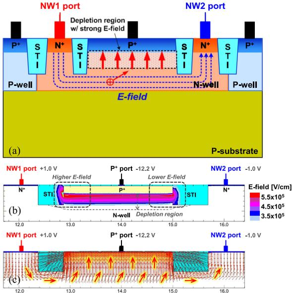
Fig. 23. (a) Movement of photogenerated carriers in N-well with an extrinsic electric field inside the charge-neutral N-well region. (b) Simulated electric field profile and (c) electric field lines of the CMOS-APD. 1.0 V and  $-1.0$  V bias voltages are applied to NW1 and NW2 ports, respectively, at the reverse bias voltage of 12.2 V for the  $P^+$ /N-well junction [41].
