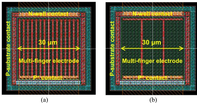
Fig. 18. Simplified CMOS-APD layouts with (a)  $1.3 \mu\text{m}$  and (b)  $9.6 \mu\text{m}$  spacing multi-finger electrodes on  $30 \times 30 \mu\text{m}^2$  optical windows.
