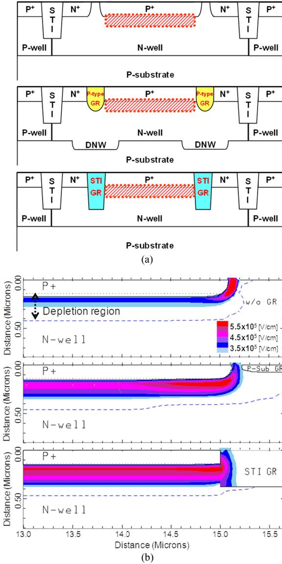
Fig. 9. (a) Cross sections and (b) simulated electric-field profiles of CMOS-APDs: (i) w/o GR, (ii) w/ P-type GR, and (iii) w/ STI GR [38].
