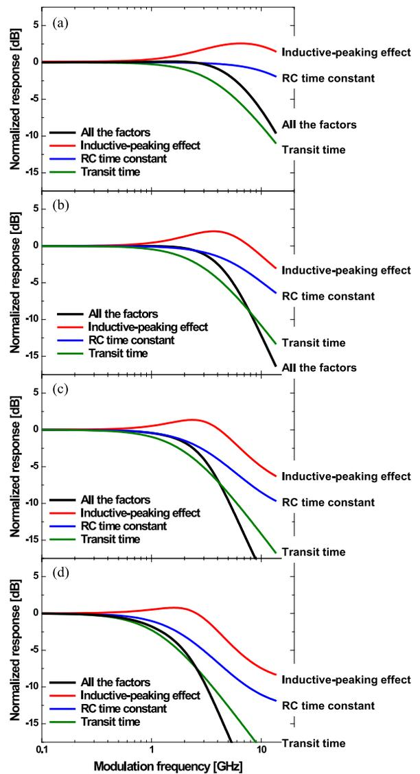
Fig. 14. Normalized photodetection frequency responses of CMOS-APDs for the photogenerated-carrier transit time, the RC time constant, the inductive-peaking effect, and all the factors according to device areas [39]. (a)  $10 \times 10 \mu\text{m}^2$ , (b)  $20 \times 20 \mu\text{m}^2$ , (c)  $30 \times 30 \mu\text{m}^2$  and (d)  $40 \times 40 \mu\text{m}^2$ .
