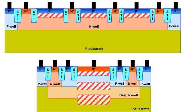
Fig. 25. Cross sections of (a) lateral and (b) vertical multi-junction CMOS-APDs.
