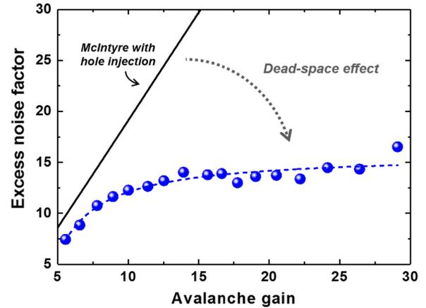
Fig. 8. Excess noise factor of a  $P^+/N$ -well CMOS-APD as a function of avalanche gain. The solid line indicates the prediction of McIntyre's model in the case of hole injection.
