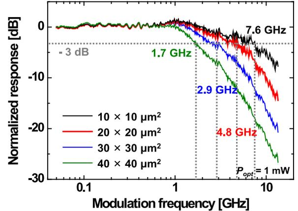
Fig. 13. Normalized photodetection frequency responses of CMOS-APDs having different device areas [39].
