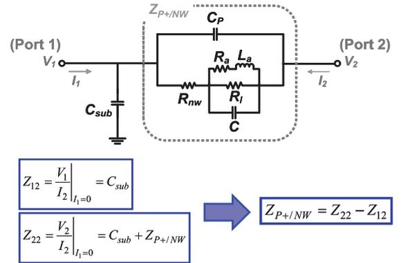
Fig. 3. Parameter extraction for the CMOS-APD equivalent circuit model.
