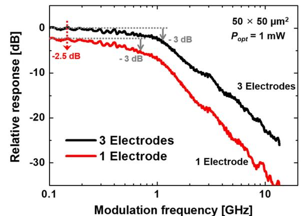
Fig. 20. Measured photodetection frequency responses of CMOS-APDs having (a) three electrodes and (b) only one electrode on optical windows.
