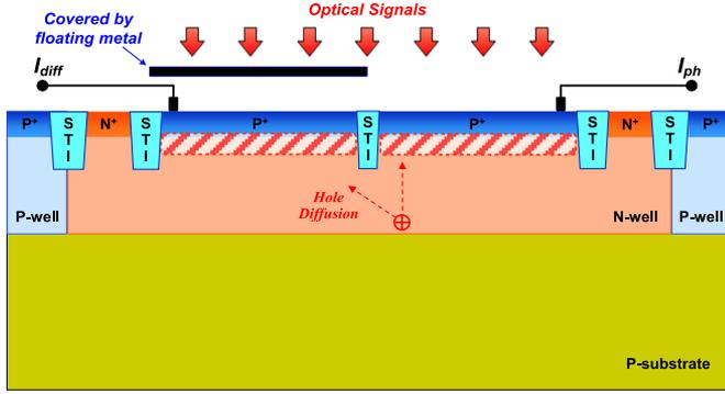
Fig. 21. Cross section of SM-APDs based on the  $P^+/N$ -well junction [43].
