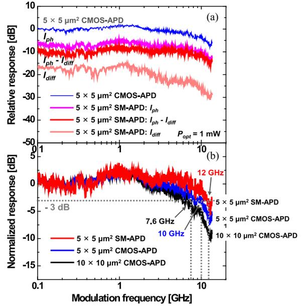
Fig. 22. (a) Measured photodetection frequency responses of the  $5 \times 5 \mu\text{m}^2$  CMOS-APD and SM-APD. (b) Normalized photodetection frequency responses of the APDs [43].
