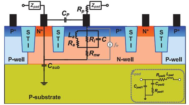
Fig. 2. Equivalent circuit model of CMOS-APDs based on the P<sup>+</sup>/N-well junction [42].
