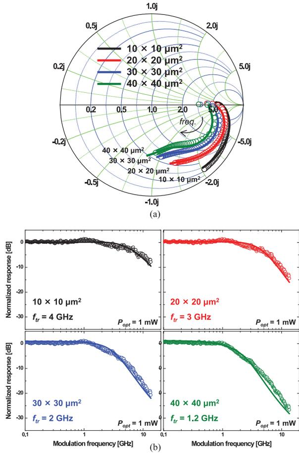
Fig. 4. (a) Measured and simulated electrical reflection coefficients and (b) photodetection frequency responses for different CMOS-APDs. Hollow circles represent the measured data and solid lines as the simulated results [39].
