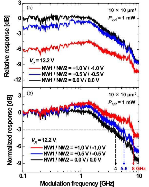
Fig. 24. (a) Relative and (b) normalized photodetection frequency responses of the CMOS-APD with different bias voltages applied to N-well [41].
