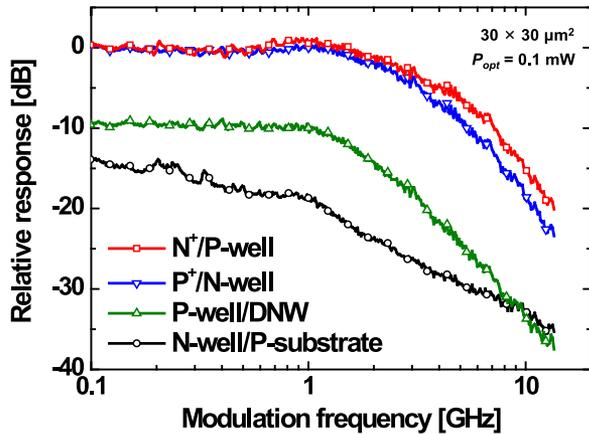
Fig. 6. Relative photodetection frequency responses of CMOS-APDs realized with different PN junctions.
