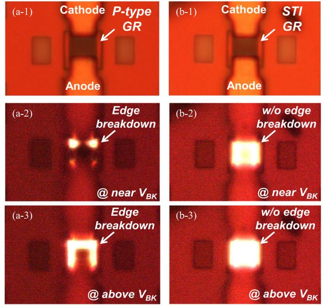
Fig. 10. Light emission tests of the fabricated CMOS-APDs: (a) w/ P-sub GR and (b) w/ STI GR.
