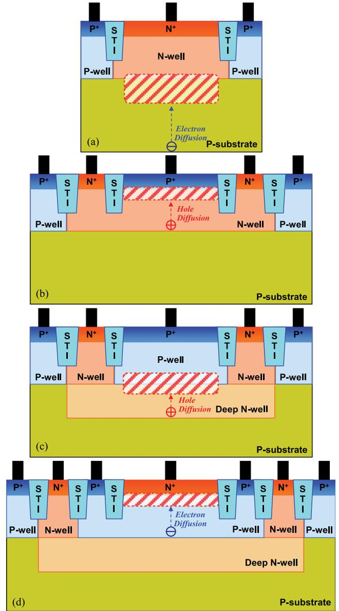
Fig. 5. Cross sections of CMOS-APDs: (a) N-well/P-substrate, (b) P<sup>+</sup>/N-well, (c) P-well/DNW, and (d) N<sup>+</sup>/P-well CMOS-APDs.
