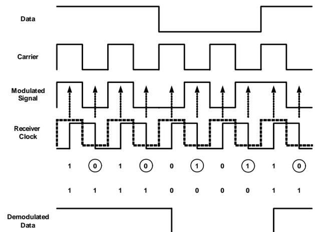
Figure 7. Proposed demodulating scheme
