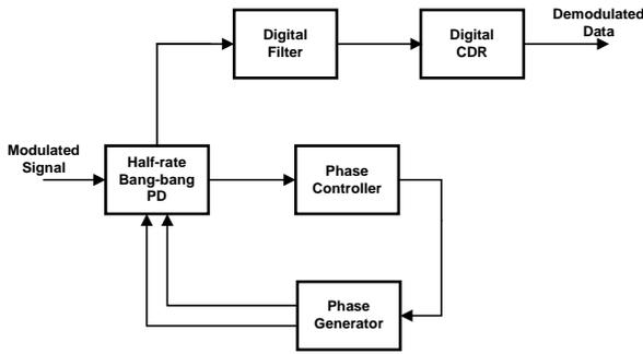
Figure 8. Block diagram of the proposed demodulator
