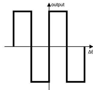
Figure 6. Characteristic of half-rate bang-bang PD
