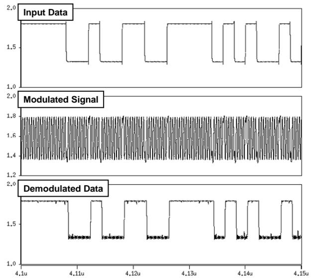
Figure 12. Simulation result : Demodulation
