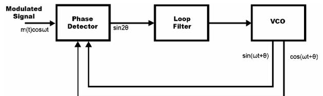
Figure 4. Modified block diagram of a Costas-loop
