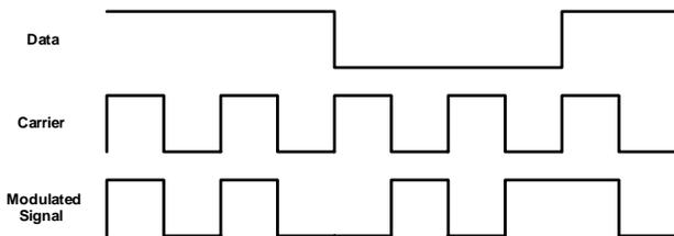
Figure 2. BPSK modulation
