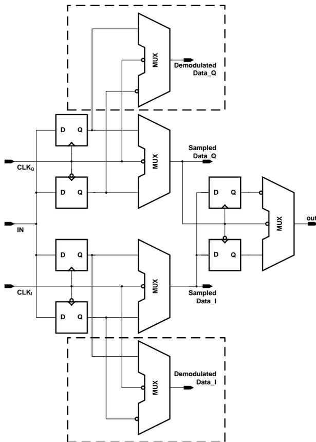
Figure 9. Modified half-rate bang-bang PD
