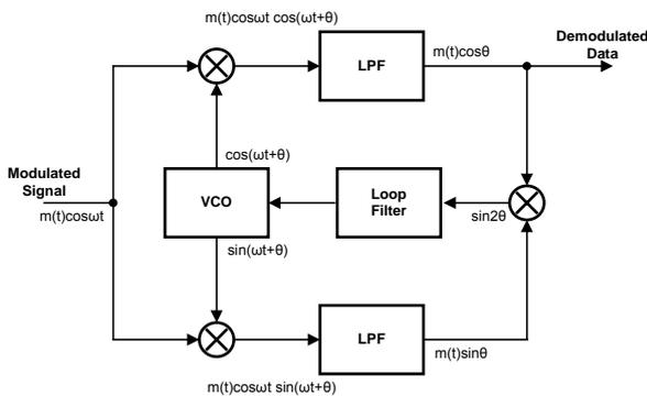
Figure 3. Block diagram of a Costas-loop
