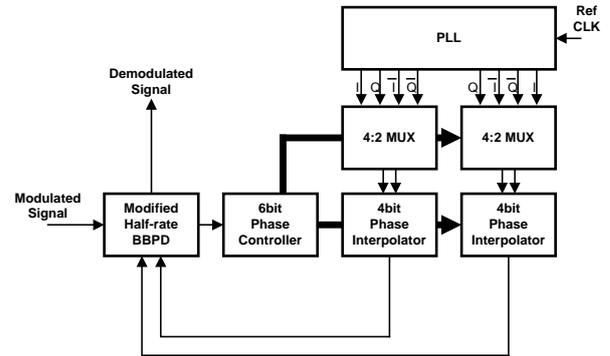
Figure 10. Block diagram of the test demodulator
