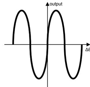
Figure 5. Characteristic of Costas-loop as a PD
