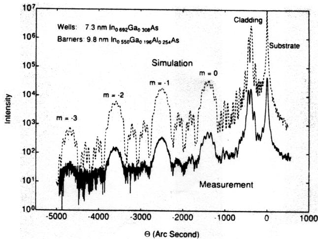
FIG. 2. Measured and simulated HRXRD scans of sample A. The input parameters for simulation that are determined from the analysis are shown in the figure.
