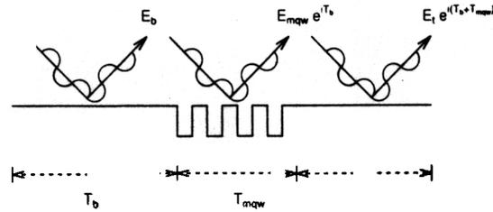
FIG. 3. Schematic diagram for separating an embedded strained MQW structure into three different regions: bottom cladding, wells and barriers, and top cladding. Notice that  $T_{MQW}$  is defined as the thickness of four wells and four barriers.
