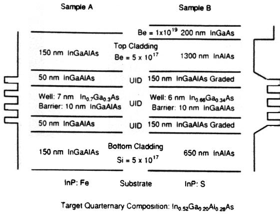
FIG. 1. Layer structures for samples A and B with target compositions and thicknesses. All the InGaAlAs quaternary layers have the same target compositions as shown in the figure. The GRINSCH layers in sample B are linearly graded from In<sub>0.52</sub>Al<sub>0.48</sub>As to In<sub>0.52</sub>Ga<sub>0.20</sub>Al<sub>0.28</sub>As. InGaAs and InAlAs layers have the lattice matching target compositions, In<sub>0.53</sub>Ga<sub>0.47</sub>As and In<sub>0.52</sub>Al<sub>0.48</sub>As, respectively.
