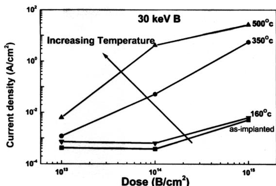
Fig. 4. Plots of B ion dose versus the average current leakage of the B implanted diodes at a reverse bias of  $-40$  V. The samples were implanted with three doses of  $1 \times 10^{13}$ ,  $1 \times 10^{14}$  and  $1 \times 10^{15}$   $\text{cm}^{-2}$  and then annealed for 30 min in  $\text{N}_2$  ambient. ( $T_1$ ) room temperature, ( $T_2$ )  $160^\circ\text{C}$ , ( $T_3$ )  $350^\circ\text{C}$  and ( $T_4$ )  $500^\circ\text{C}$ .
