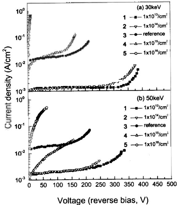
Fig. 2. Reverse current–voltage ( $I$ – $V$ ) characteristics for an unimplanted Au/n-Si Schottky diode (curve 3) and the diodes implanted to doses of  $1 \times 10^{13}$  (curve 1),  $1 \times 10^{14}$  (curve 2),  $1 \times 10^{15}$  (curve 4),  $1 \times 10^{16}$   $\text{cm}^{-2}$  (curve 5) with the implantation energies of (a) 30 and (b) 50 keV.
