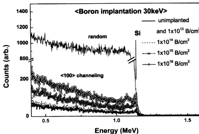
Fig. 3. The 2 MeV  ${}^4\text{He}^{2+}$  (100) channeling spectra for unimplanted sample and samples implanted to different doses of  $1 \times 10^{13}$ ,  $1 \times 10^{14}$ ,  $1 \times 10^{15}$  and  $1 \times 10^{16}$   $\text{cm}^{-2}$  with an implantation energy of 30 keV.
