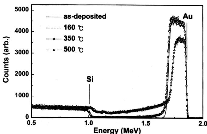
Fig. 5. The 2 MeV  $^4\text{He}^{2+}$  backscattering spectra for test samples of 120 nm-thick Au on a unimplanted n-type Si. Those samples were annealed at an  $\text{N}_2$  ambient for 30 min.
