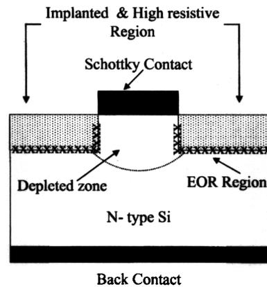
Fig. 1. Cross-sectional view of a Au/n-Si Schottky diode implanted with boron ions for edge termination.
