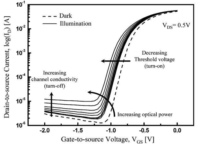
Fig. 3. Drain currents ( $I_D$ ) as a function of gate-to-source voltages ( $V_{\text{GS}}$ ) for the InP HEMT under dark and illuminated conditions at the drain-to-source voltage ( $V_{\text{DS}}$ ) of  $0.5 \text{ V}$ . The incident optical powers increases from  $-6$  to  $15 \text{ dBm}$  with the step of  $3 \text{ dB}$ .
