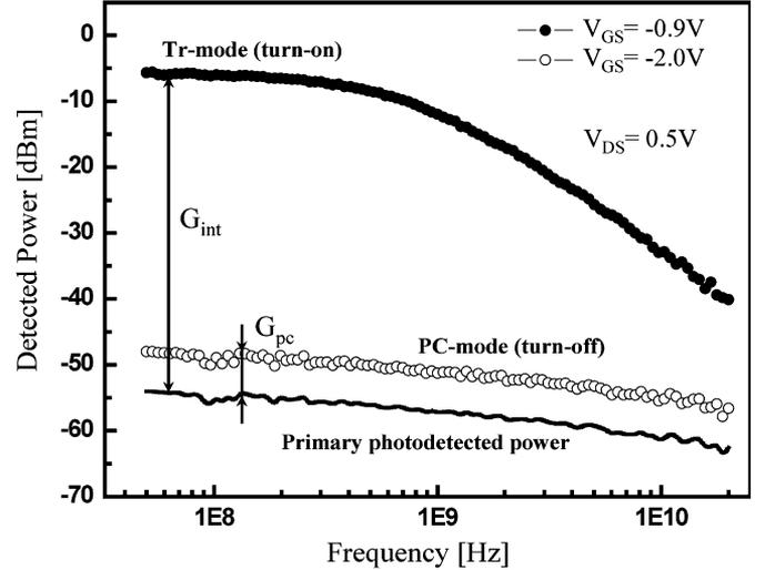
Fig. 5. Measured optical modulation response of the InP HEMT under  $V_{GS}$  of  $-0.9$  V (turn-on) and  $-2$  V (turn-off) at fixed  $V_{DS}$  of 0.5 V. The solid line is the primary photodetected power extracted from measured data at the turn-off state.  $G_{int}$  and  $G_{pc}$  represent the phototransistor internal gain and photoconductor gain, respectively.
