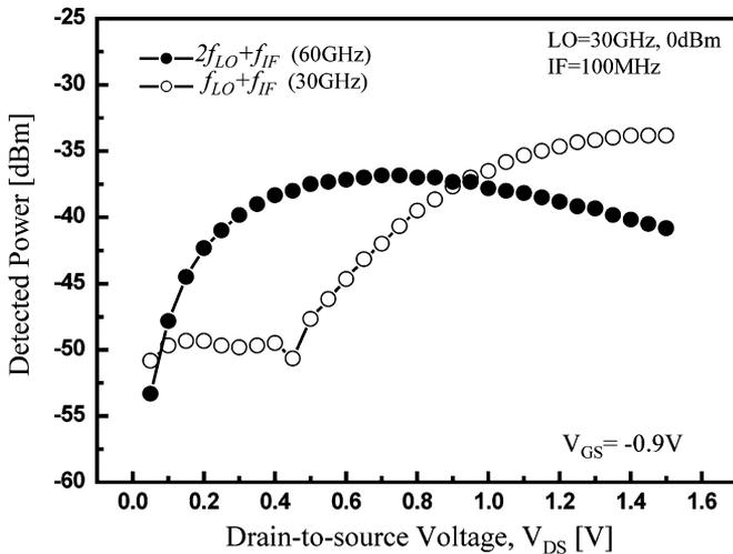
Fig. 8. Dependence of optoelectronic up-converted signals at  $f_{LO} + f_{IF}$  and  $2f_{LO} + f_{IF}$  on  $V_{DS}$  under application of a 30-GHz 0-dBm LO and 100-MHz optical IF signals at  $V_{GS} = -0.9$  V.
