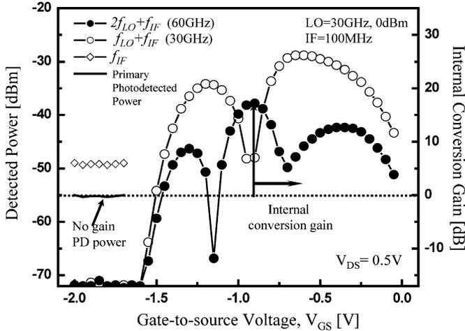
Fig. 7. Dependence of optoelectronic up-converted signals at  $f_{LO} + f_{IF}$  and  $2f_{LO} + f_{IF}$  on  $V_{GS}$  under application of a 30-GHz 0-dBm LO to the gate port and 100-MHz optical IF signals at  $V_{DS}$  of 0.5 V. The solid line indicates the primary photodetected power extracted from measured data at the turn-off state. The internal conversion gain defined as the ratio of output up-converted signal powers to the primary photodetected power is also included.
