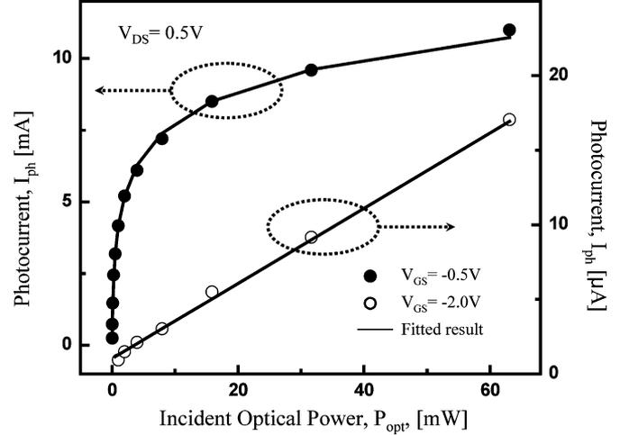
Fig. 4. Photocurrent as a function of incident optical power to the HEMT under turn-on ( $V_{GS} = -0.5$  V) and turn-off ( $V_{GS} = -2$  V) states. The symbols are measured data and solid lines are fitted results according to (1) and (2).
