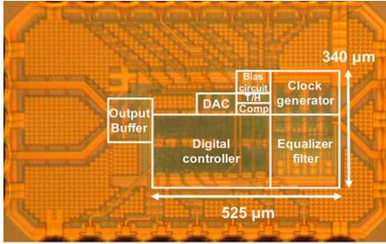
Fig. 6. Die photographs of prototype adaptive CTLE.
