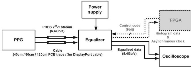
Fig. 7. Measurement setup.
