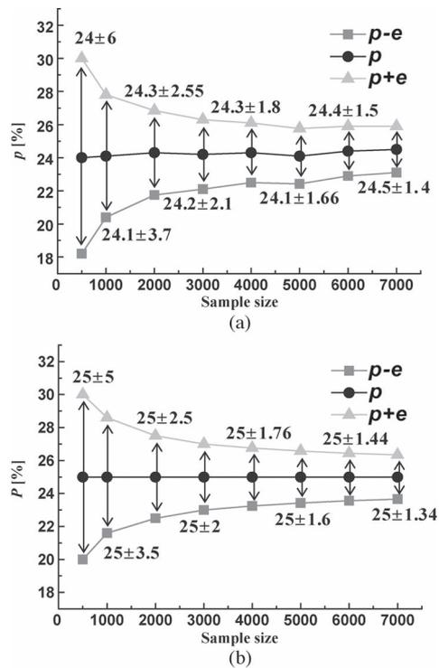
Fig. 10. (a) Measured  $p$  and  $e$  of 40-cm PCB trace and (b) calculated  $p$  and  $e$  for different sample sizes.
