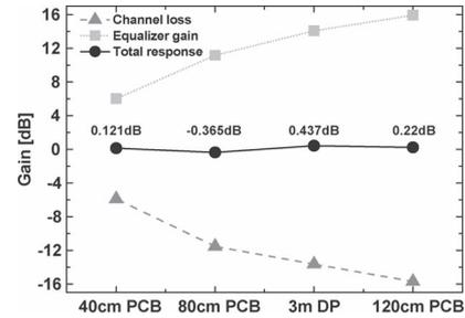
Fig. 3. Channel losses and corresponding optimal equalizer gains.
