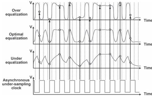
Fig. 1. Asynchronous undersampling process.
