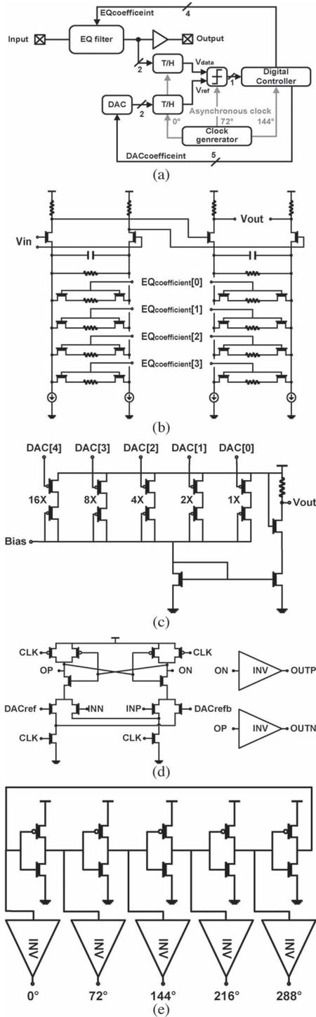
Fig. 4. (a) Block diagram of adaptive CTLE and schematics of (b) equalizing filter, (c) 5-bit DAC, (d) comparator, and (e) clock generator.
