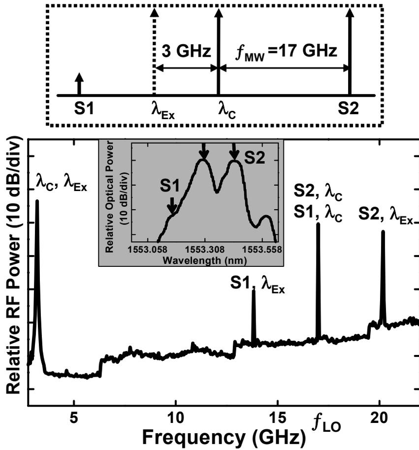
Figure 5.6 Measured optical spectra for SSB after FP-LD (b).
