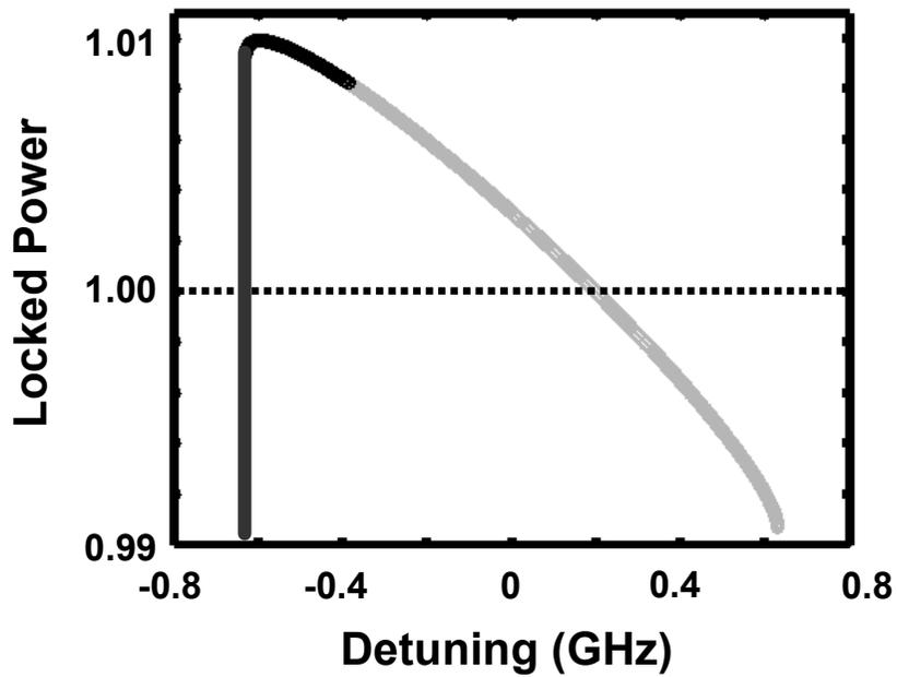
**Figure 3.3 Locked power relative to free running power. Dark solid line and light solid line represent the dynamically stable locking states and unstable locking states, respectively**
