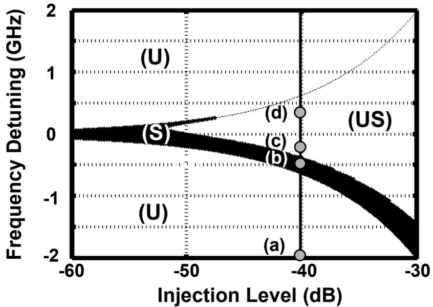
Figure 3.2 Locking characteristics as a function of injection level. S represents dynamically stable locking range; US dynamically unstable locking range; and U static unlocking range.
