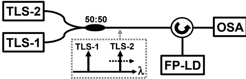
**Figure 4.3 Experimental setup for characteristics of the SL under two ML light injections. TLS: tunable light source and OSA: optical spectrum analyzer,**
