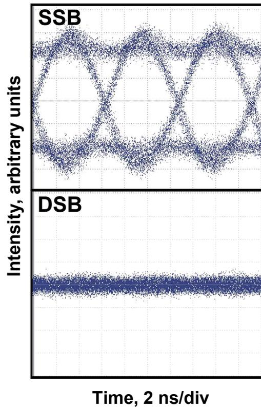
**Figure 5.8** Received eye diagrams of 155 Mb/s data signal at the received optical power of 7.8 dBm for DSB signal before FP-LD and for SSB signal after FP-LD.
