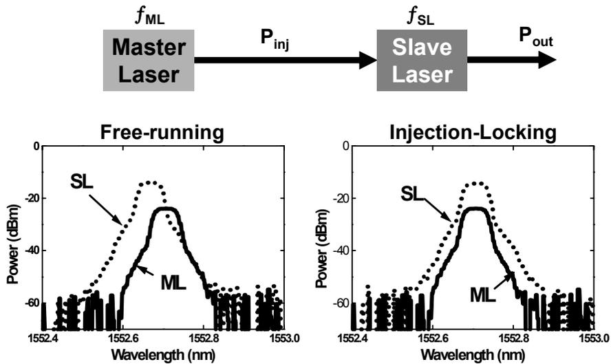
Figure 3.1 Optical injection locking configuration.
