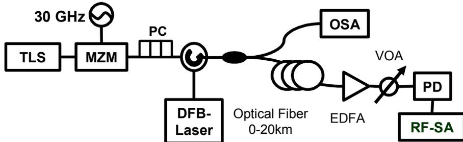
**Figure 5.2** Experimental setup for optical single sideband modulation. **TLS:** tunable light source, **MZM:** Mach-Zehnder intensity modulator, **PC:** polarization controller; **OSA:** optical spectrum analyzer, **EDFA:** erbium-doped fiber amplifier, **VOA:** variable optical attenuator, and **RF-SA:** RF-spectrum analyzer.
