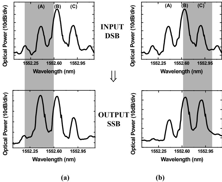
**Figure 5.3 Measured optical spectra for input DSB and output optical SSB for the case that one mode of DSB at shorter wavelength (A) is within locking range (a) and for the case that two modes of DSB (B and C) are within locking range (b).**
