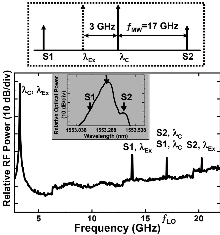
Figure 5.6 Measured optical spectra for DSB before FP-LD (a).
