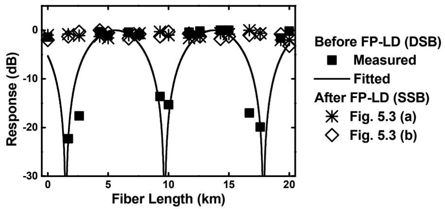
Figure 5.4 Measured RF power versus fiber length
