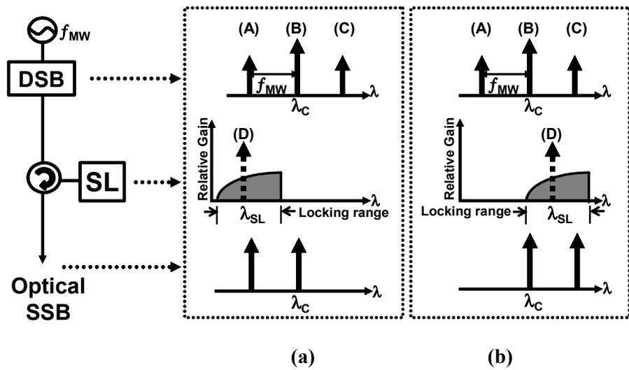
**Figure 5.1 Proposed schemes. (a) For the case in which one mode of DSB (A) at the shorter wavelength is within locking range. (b) For the case in which two modes of DSB (B and C) at the longer wavelength are within locking range. SL: Semiconductor laser.**
