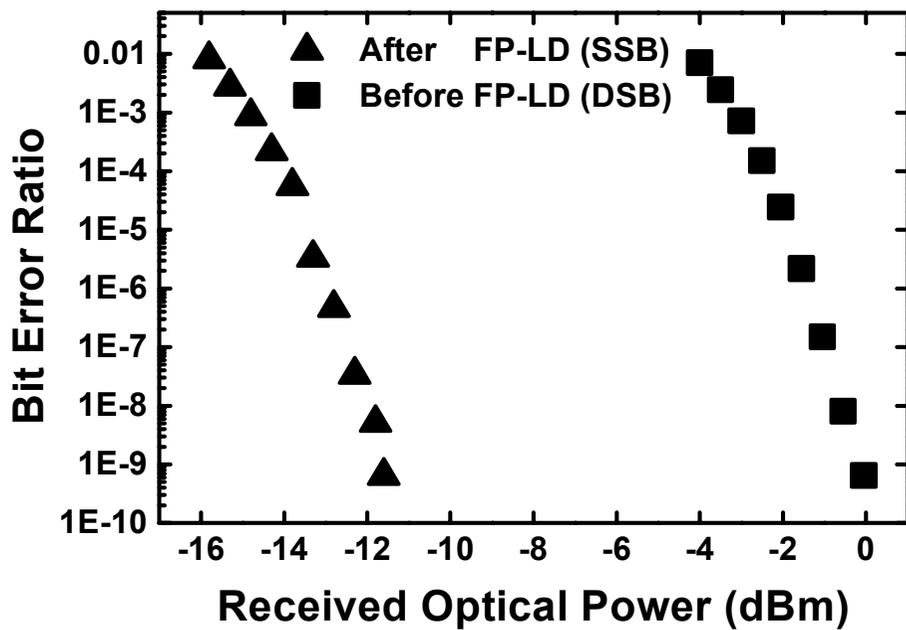
**Figure 5.7 Measured Bit Error Rate versus received optical power for DSB signal before FP-LD and for SSB signal after FP-LD.**
