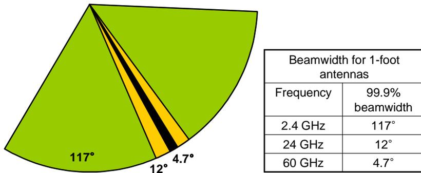
Figure 1-2. Directivity comparison among ISM band carrier signals.
