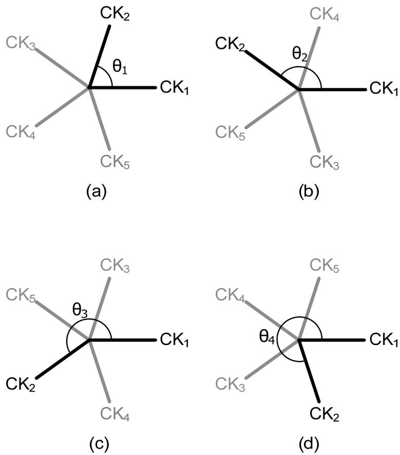
Figure 2-3. Four  $\theta$ s of a five-stage RO.
