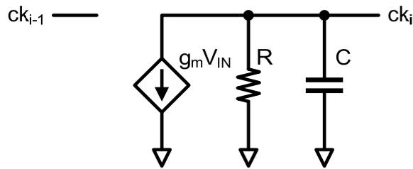
Figure 2-7. A small signal equivalent circuit of an inverter
