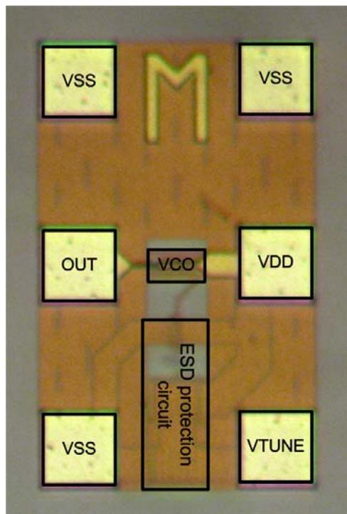
Figure 4-7. Microphotograph of the implemented five-stage FRO.
