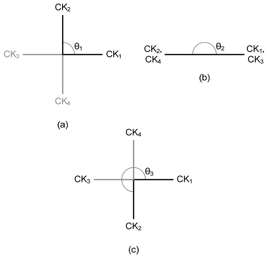
Figure 3-3. Possible oscillation modes of four-stage FRO. (a) Mode 1,  $\theta = \pi/2$ . (b) Mode 2,  $\theta = \pi$ . (c) Mode 1,  $\theta = 3\pi/2$ .
