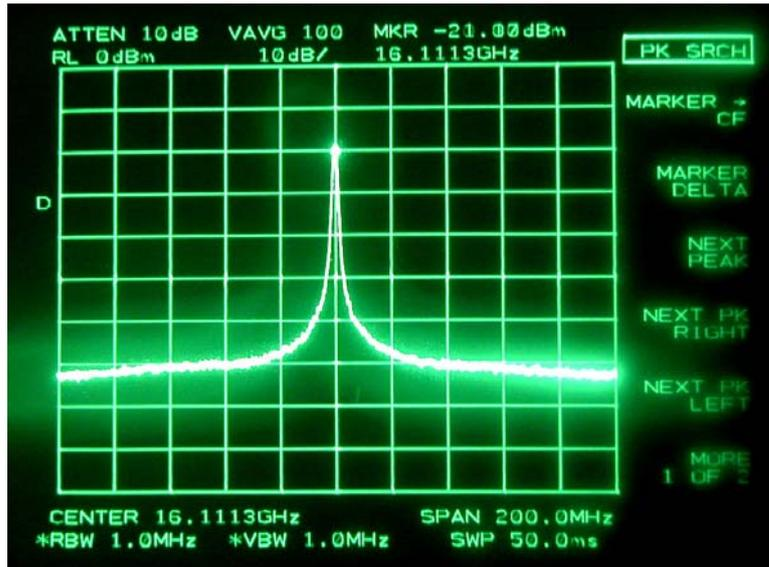
Figure 4-9. Output spectrum of the FRO at 16GHz.
