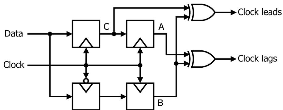
Figure 6-1. A schematic diagram of bang-bang PD
