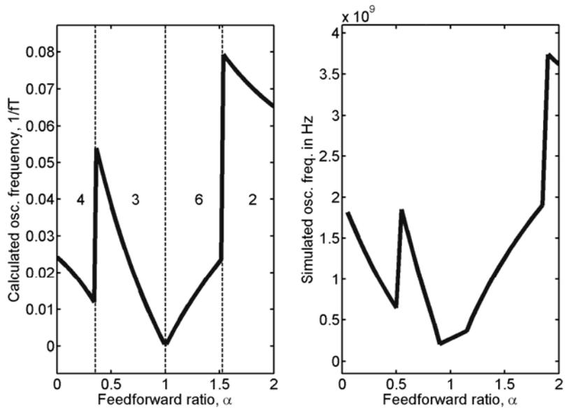
Figure 3-14. Calculated and simulated oscillation frequency of nine-stage CMOS FRO.
