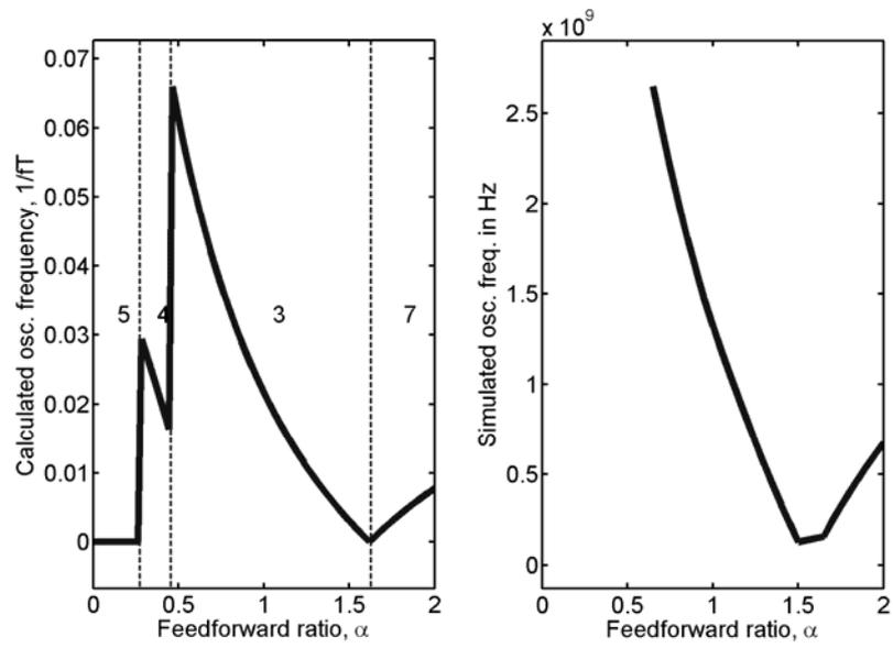
Figure 3-15. Calculated and simulated oscillation frequency of ten-stage CMOS FRO.
