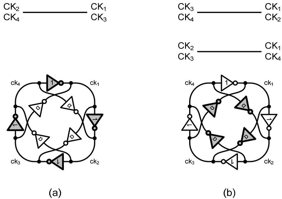
Figure 3-5. Two types of latch up
