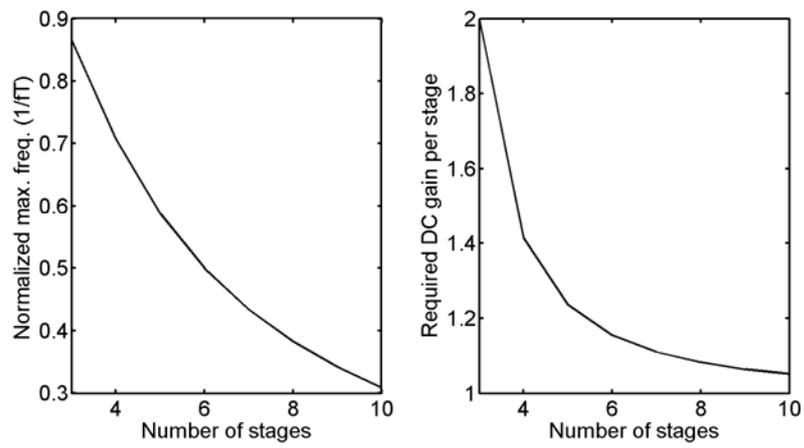
Figure 1-5. Maximum achievable oscillation frequency and the required minimum DC gain per delay element.
