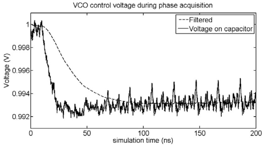
Figure 6-11. Simulated VCO control voltage during phase acquisition
