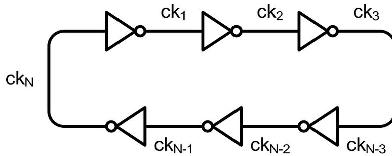
Figure 2-1. Schematic diagram of a typical N-stage CMOS SPRO.
