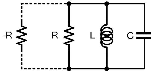
Figure 1-2. A resonator based oscillator model. Energy supplement circuit is depicted as a negative resistance.
