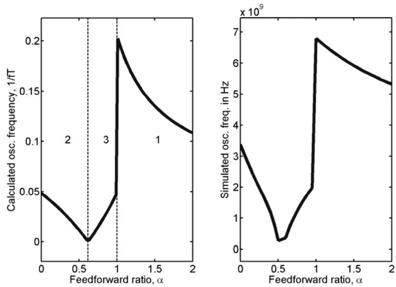
Figure 3-10. Calculated and simulated oscillation frequency of five-stage CMOS FRO.
