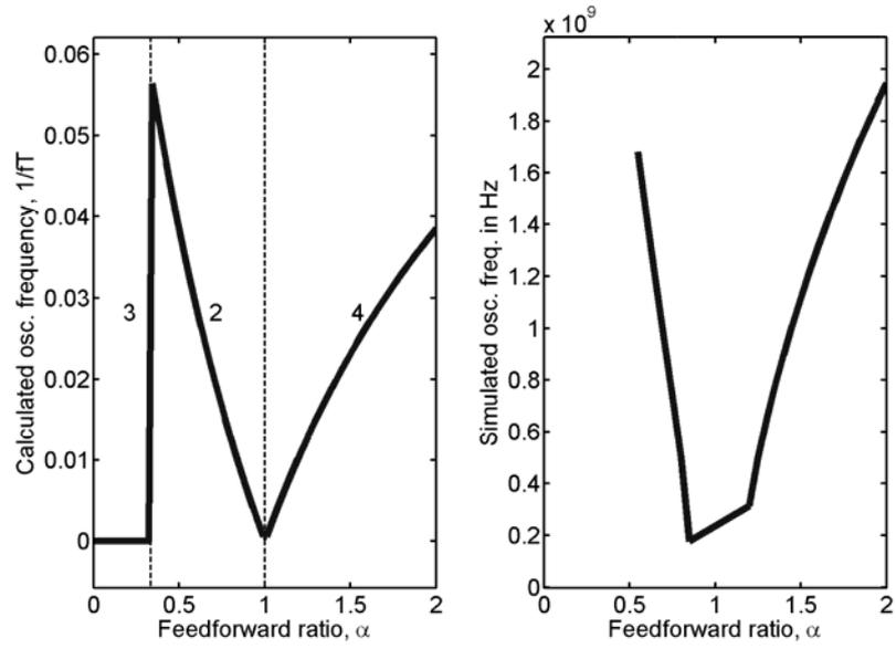
Figure 3-11. Calculated and simulated oscillation frequency of six-stage CMOS FRO.
