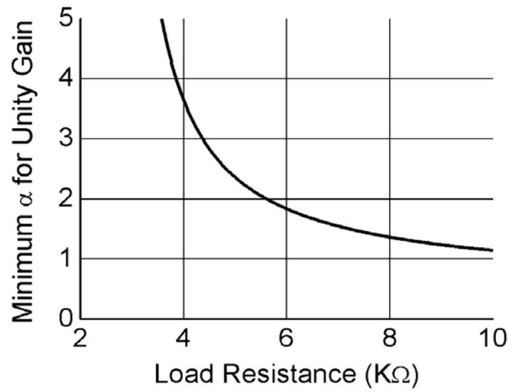
Figure 4-4. Calculated  $\alpha_{\text{MIN}}$  required for mode 1 operation
