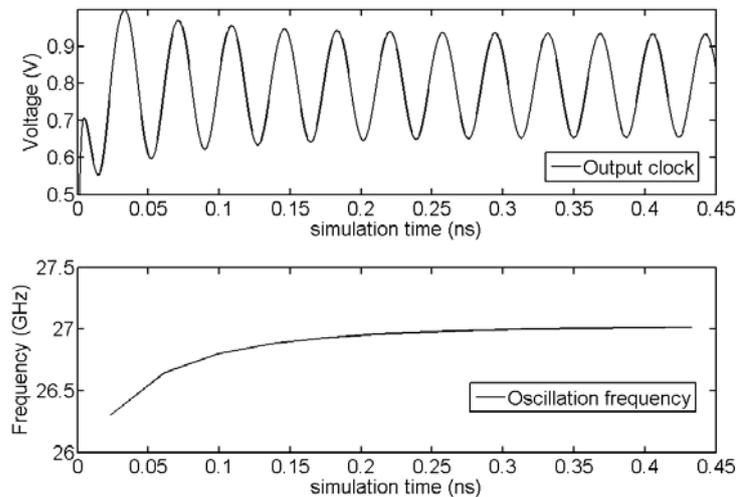
Figure 4-11. Simulation results of five-stage FRO in 65nm CMOS technology
