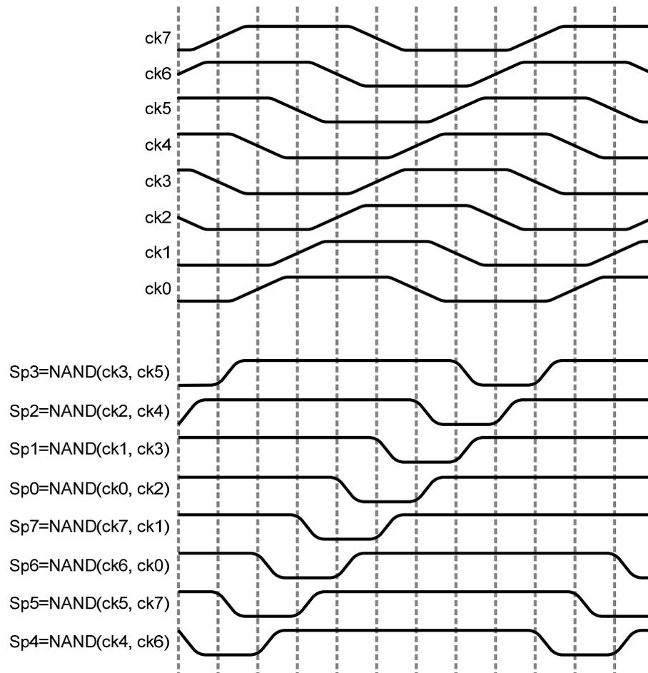
Figure 6-6. Sampling and clearing pulse generation using eight-phase clock.
