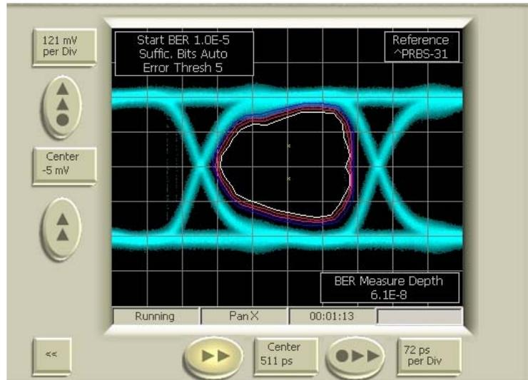
Figure 6-15. BER contour overlapped on the eye-diagram of recovered data
