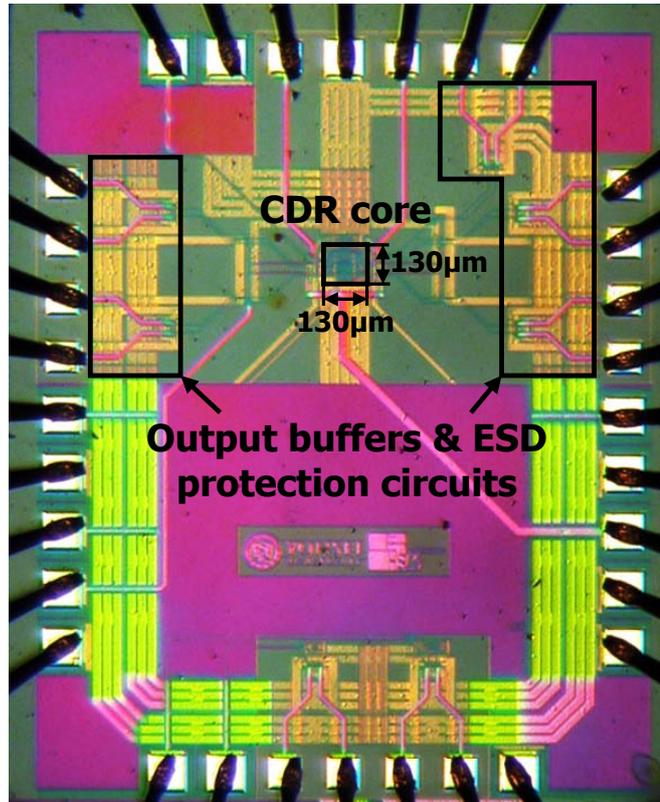
Figure 6-12. Microphotograph of fabricated CDR circuit
