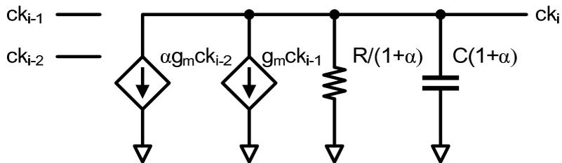
Figure 2-8. A small signal equivalent circuit of an inverter
