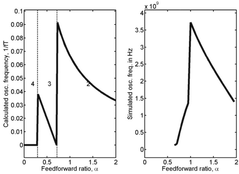
Figure 3-13. Calculated and simulated oscillation frequency of eight-stage CMOS FRO.
