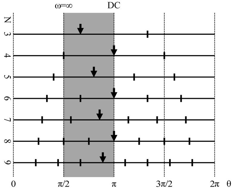
Figure 2-4. Possible oscillation modes of an inverter-based N-stage ROs (N=3~9).
