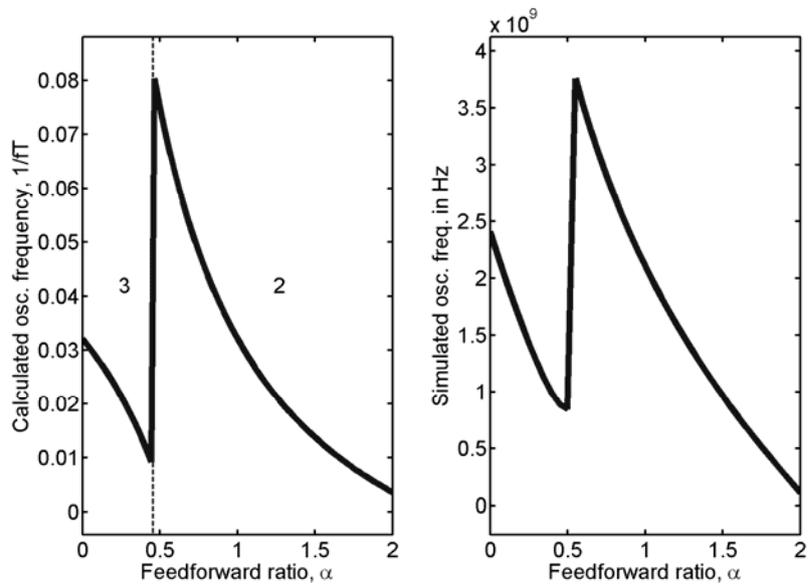
Figure 3-12. Calculated and simulated oscillation frequency of seven-stage CMOS FRO.
