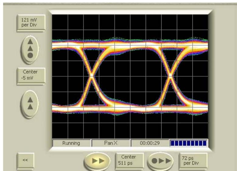
Figure 6-14. Eye-diagram of recovered data with PRBS pattern
