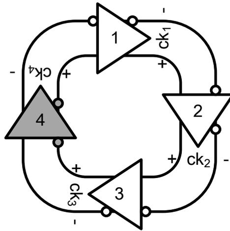
Figure 3-1. Schematic diagram of typical four-stage RO. It has differential buffer as its unit stage. The signal polarity is switched at the grey-colored stage.
