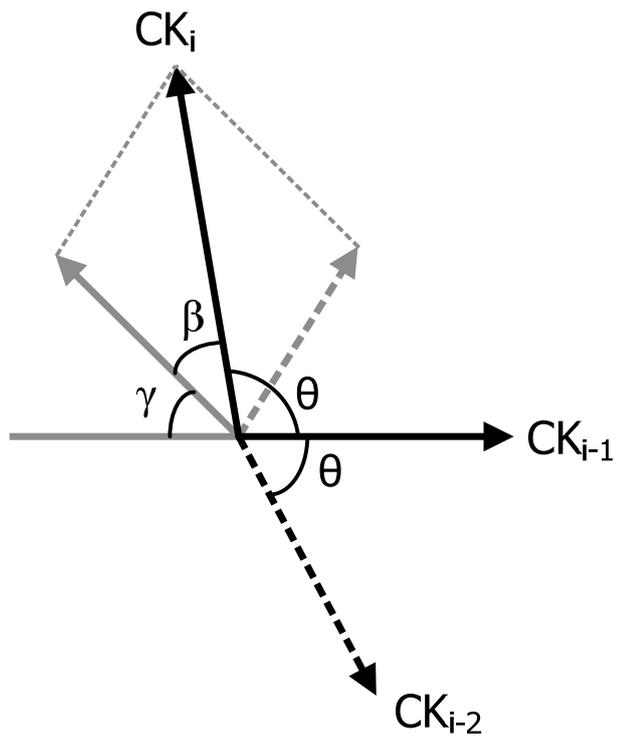
Figure 2-9. The phase relationship of the inputs and the output of the unit stage in oscillation.
