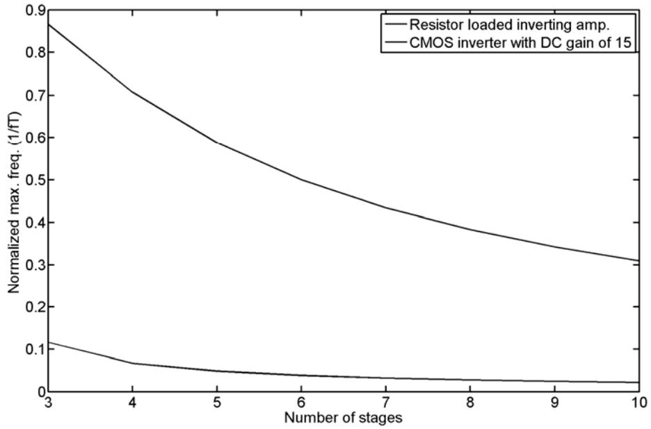
Figure 1-6. Calculated oscillation frequency of CMOS RO. The CMOS inverter's DC gain is assumed to be 15.
