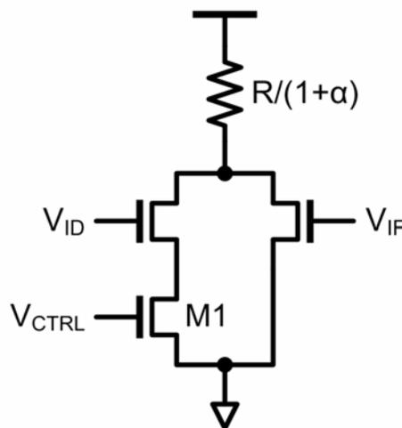
Figure 4-6. Schematic diagram of the implemented unit stage of the five-stage FRO.
