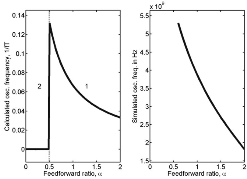
Figure 3-9. Calculated and simulated oscillation frequency of four-stage CMOS FRO.
