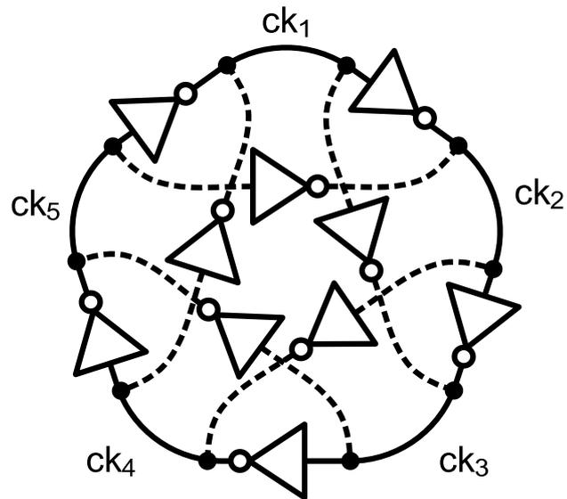
Figure 2-5. Five-stage feedforward ring oscillator
