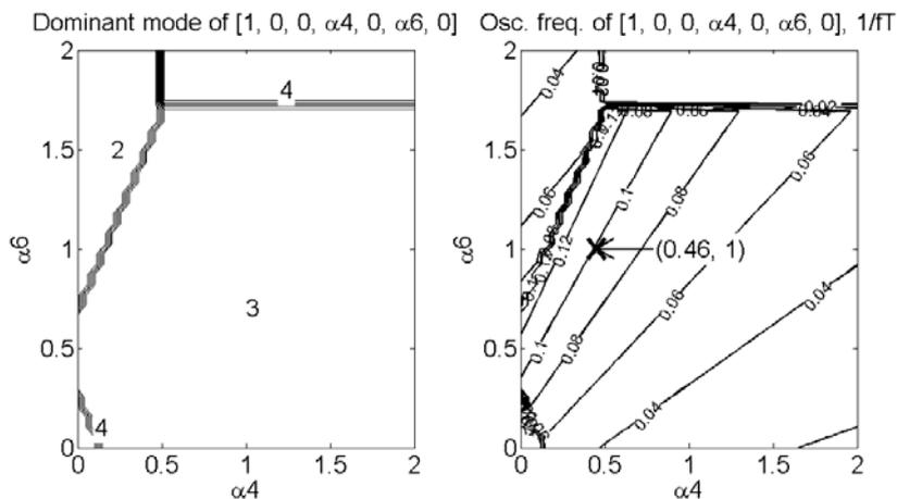
Figure 6-7. Determining feedforward ratio of eight-phase MFRO.
