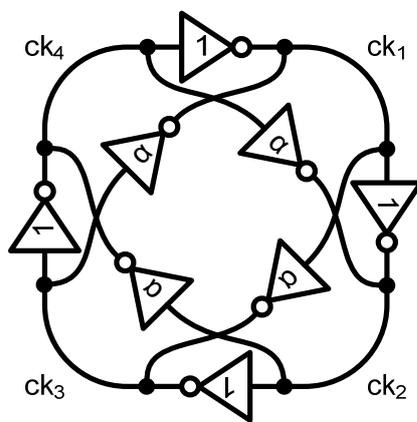
Figure 3-2. Schematic diagram of four-stage FRO.
