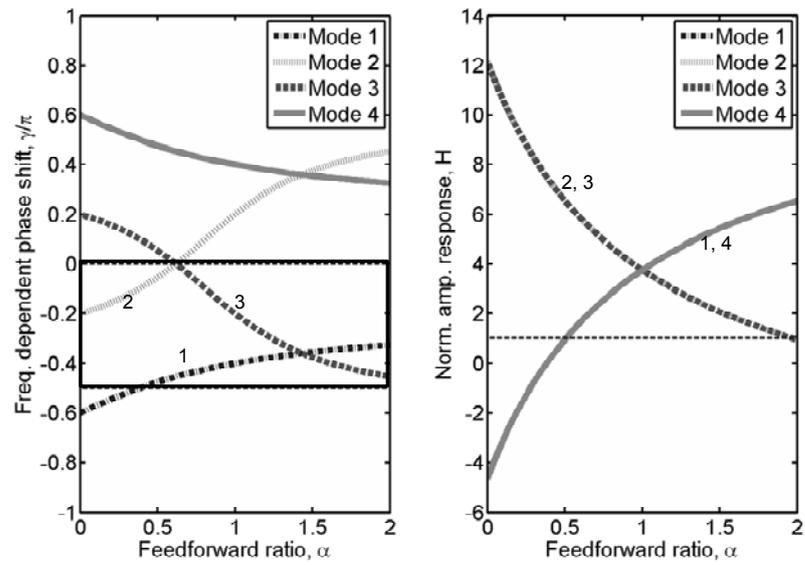
Figure 2-11. Left: The frequency dependent phase shift  $\gamma$  should be in a range between 0 and  $-\pi/2$ .
