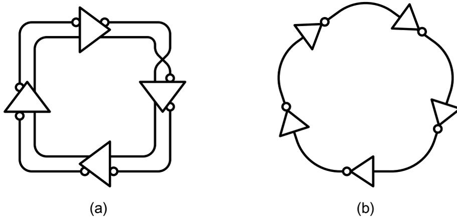
Figure 1-3. Schematic diagram of typical ROs. (a) A four-stage differential-ended RO. (b) A five-stage single-ended RO.
