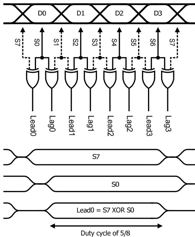
Figure 6-4. XOR array in PDs with eight-data samples
