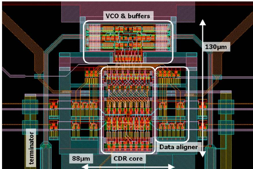
Figure 6-10. Layout close-up of designed CDR
