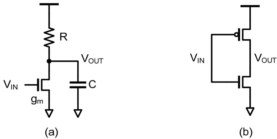
Figure 1-4. Simple first-order inverter circuits. (a) A resistor-loaded inverting amplifier with load resistance C. (b) CMOS inverter.
