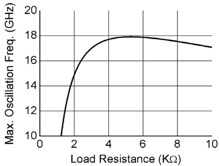
Figure 4-5. Calculated oscillation frequency
