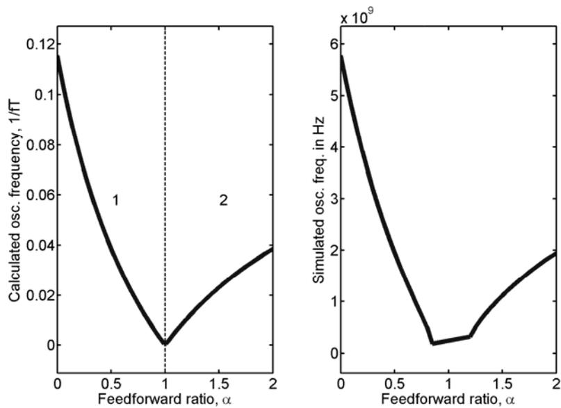
Figure 3-8. Calculated and simulated oscillation frequency of three-stage CMOS FRO.
