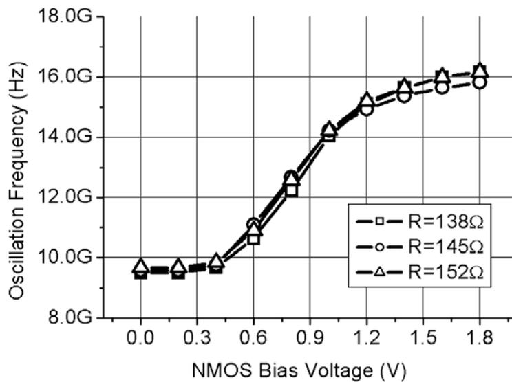
Figure 4-8. Measured oscillation frequency of the five-stage FRO.
