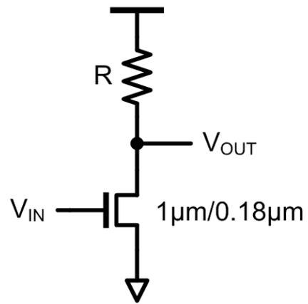
Figure 4-1. Schematic diagram of a simple inverting amplifier
