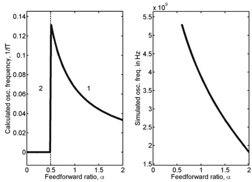
Figure 3-7. Calculated and simulated oscillation frequency of four-stage FRO.
