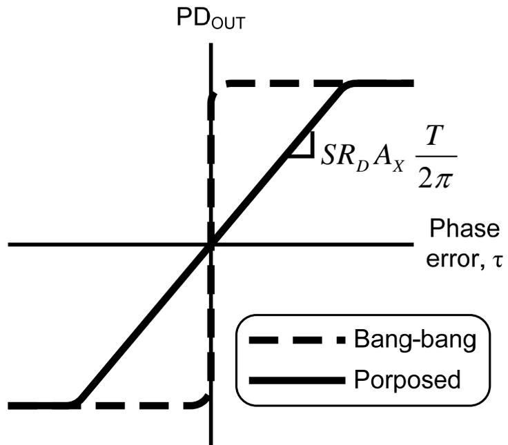
Figure 6-3. PD output response curves of proposed linear PD
