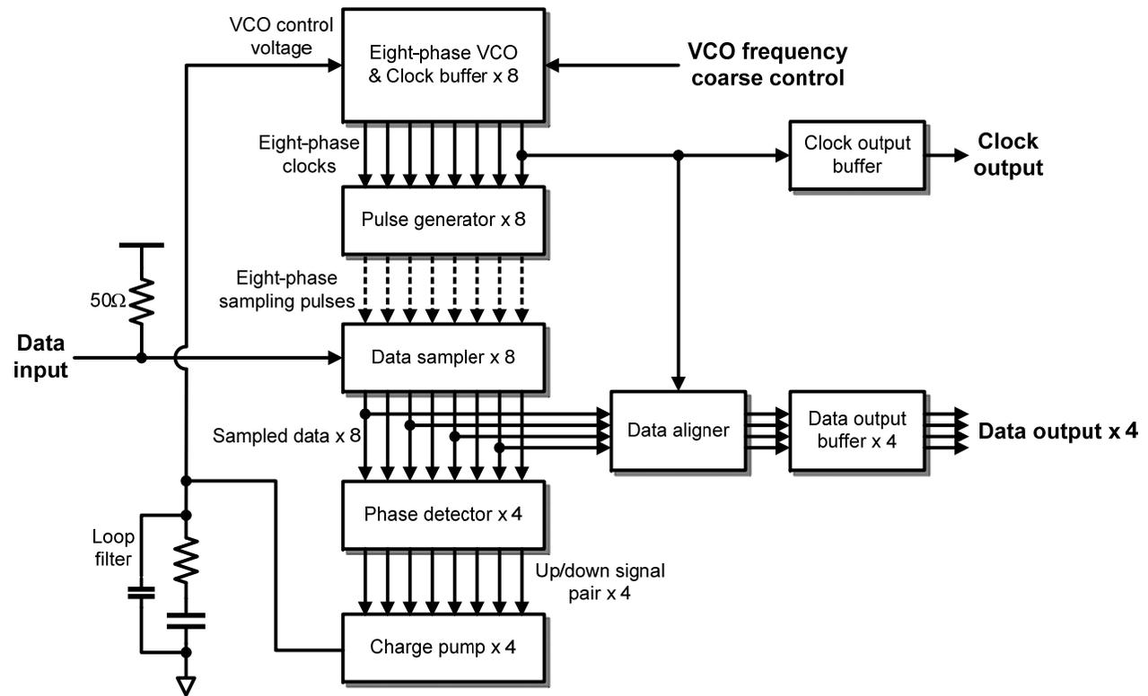
Figure 6-9. Schematic diagram of designed CDR.
