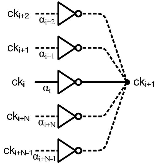
Figure 5-1. Generalized unit stage structure of MFRO.
