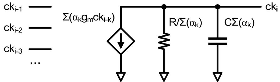
Figure 5-2. A small signal equivalent circuit of the unit stage.
