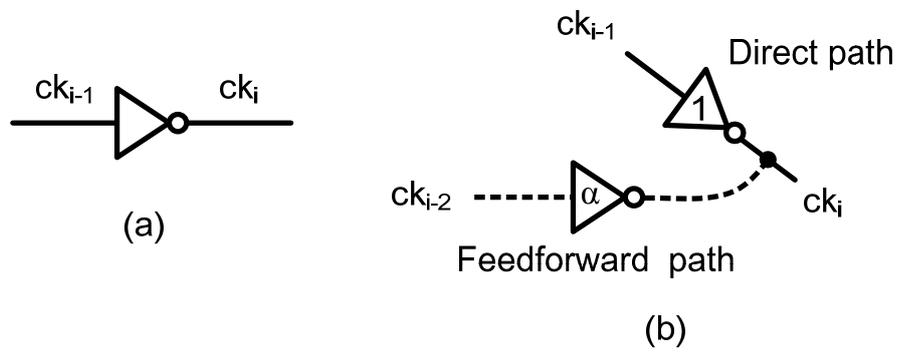
Figure 2-6. Unit stage structures. (a) Conventional single path RO. (b) Five-stage FRO.
