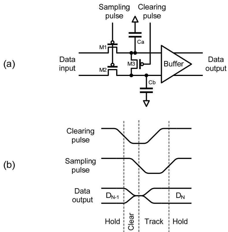
Figure 6-5. (a) Schematic diagram of data sampler. (b) Sampler operation.
