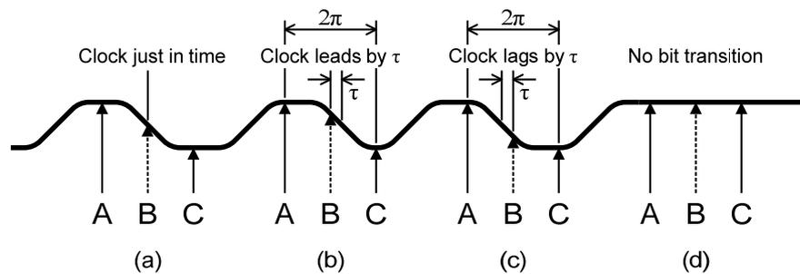
Figure 6-2. Operation of bang-bang PD
