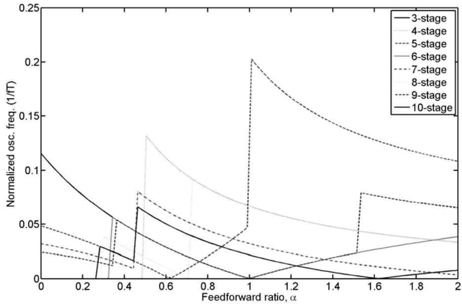
Figure 3-16. Oscillation frequency comparison of various number stage CMOS FROs.
