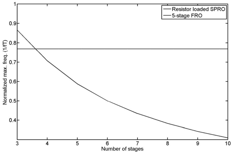
Figure 4-2. Comparison between maximum achievable oscillation frequencies of SPRO and the optimized five-stage FRO.
