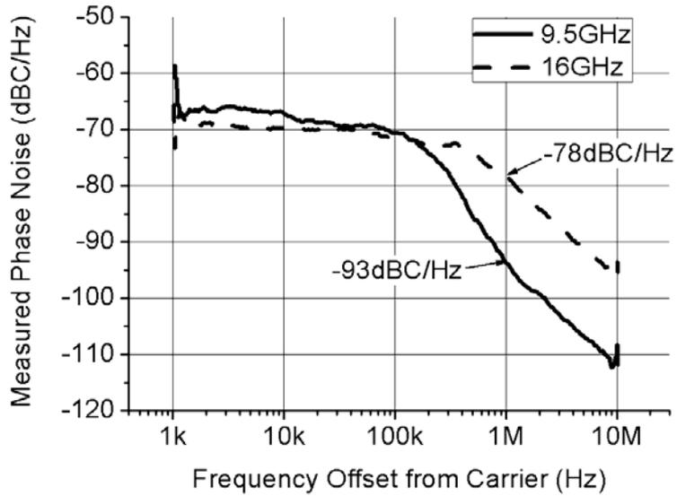
Figure 4-10. Measured output phase noise of the FRO.
