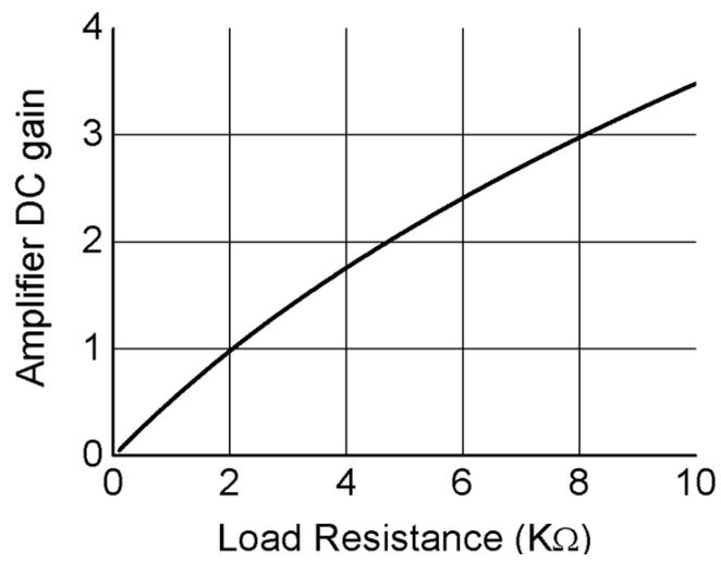
Figure 4-3. Simulated DC gain of the inverting amplifier.
