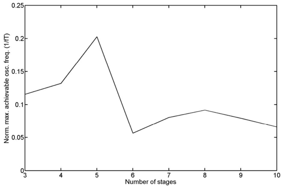
Figure 3-17. Maximum achievable oscillation frequency of CMOS FROs with N=3~10. The CMOS inverter's DC gain is 15. The oscillation frequency is normalized by f<sub>T</sub>.
