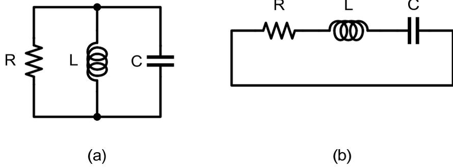
Figure 1-1. (a) Parallel RCL circuit. (b) Series RLC circuit.
