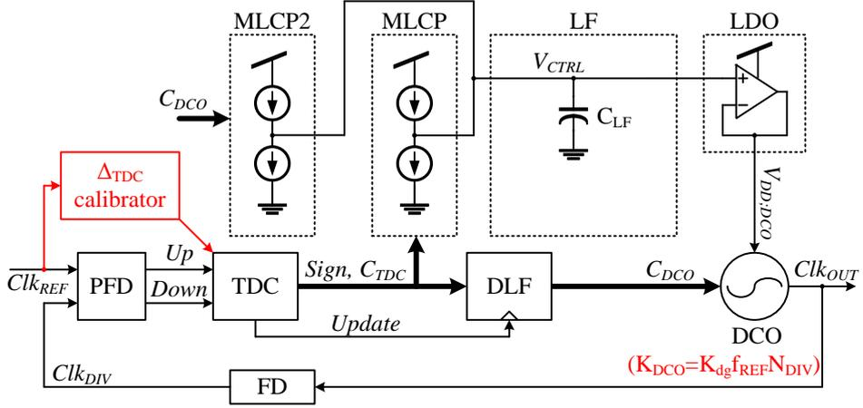
Figure 4.8: Block-diagram of secondly modified PLL
