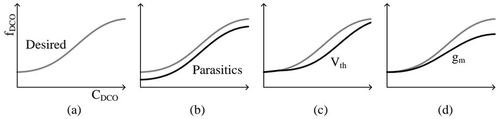
Figure 2.8: Examples of PVT-sensitive circuit parameters influencing DCO frequency curve
