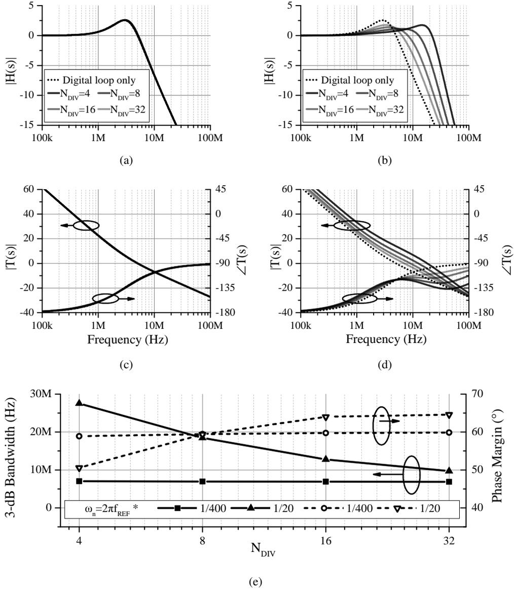
Figure 2.7: Small-signal model simulation results of proposed PLL with  $N_{DIV}$  variations, (a) closed-loop magnitude response with low  $\omega_n$  ( $=2\pi f_{REF}/400$ ), (b) with high  $\omega_n$  ( $=2\pi f_{REF}/20$ ), (c) open-loop magnitude and phase responses with low  $\omega_n$ , (d) with high  $\omega_n$ , (e) 3-dB bandwidth and phase margin variations
