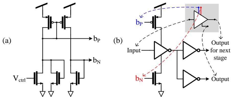
Figure 4.15: Schematics of (a) bias generator, (b) voltage-controlled delay cell
