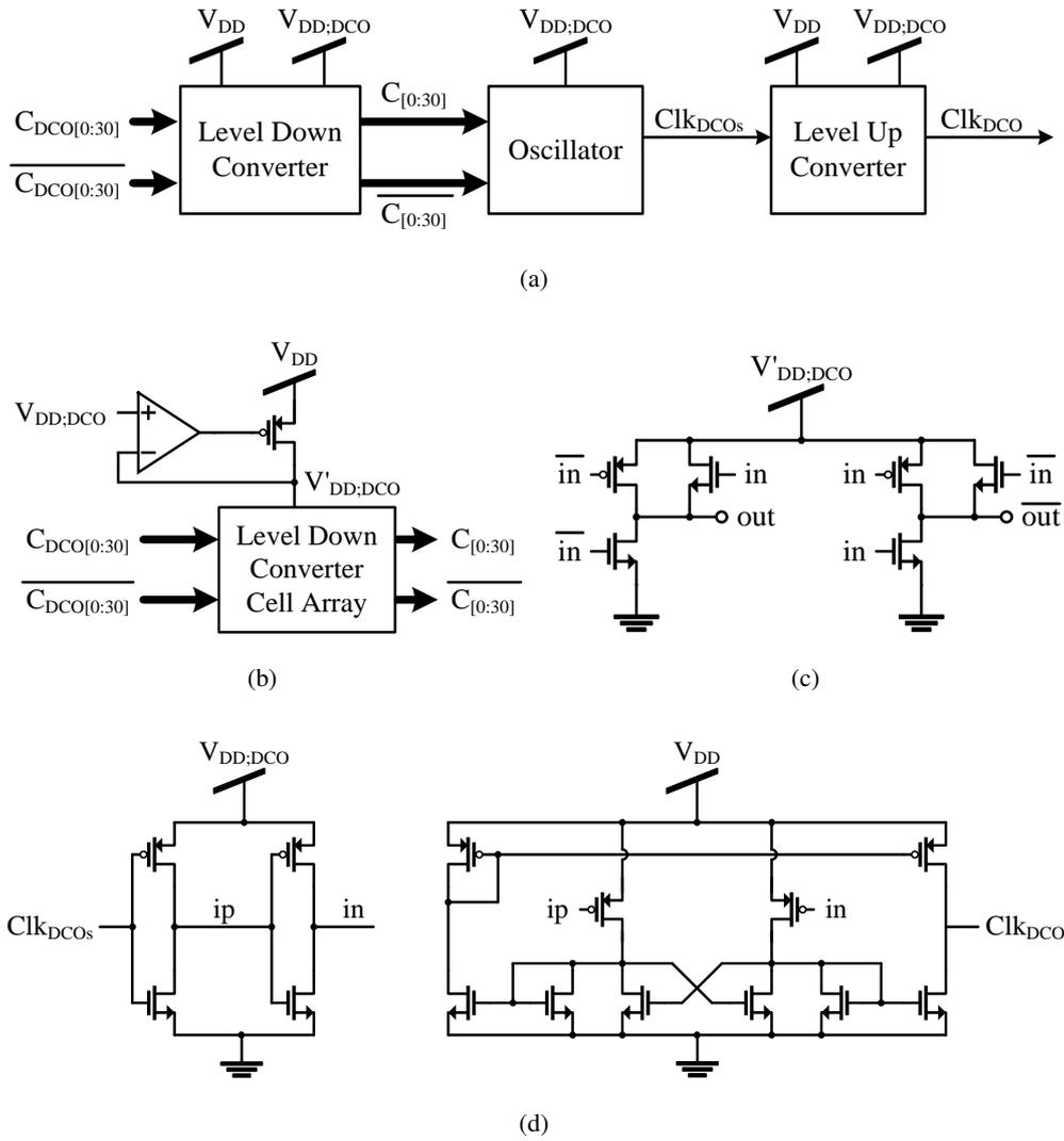
Figure 2.11: (a) Block-diagram of proposed DCO with input and output level converters, (b) level down converter, (c) schematics of level down converter cell, (d) schematics of level up converter
