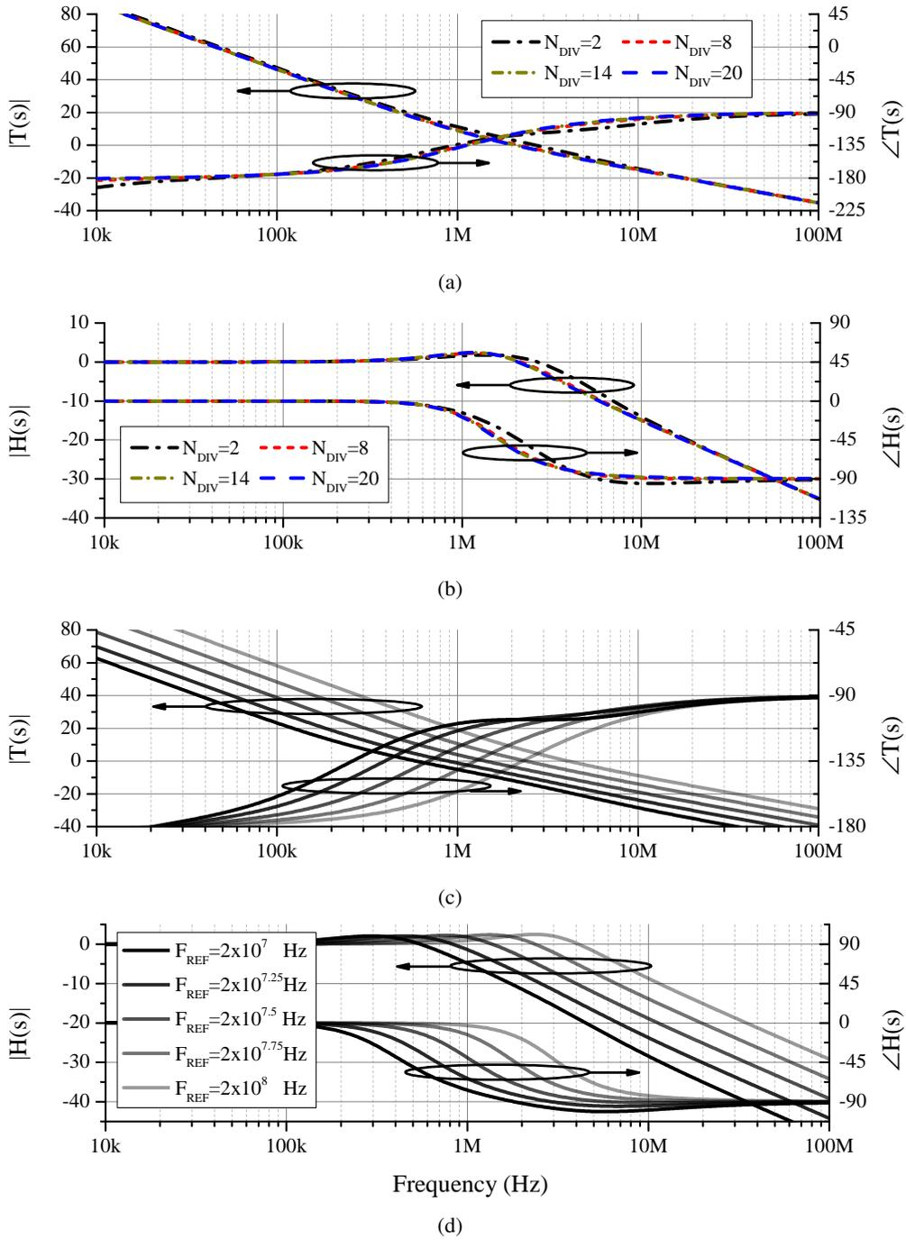
Figure 4.9: Small-signal transfer function of secondly modified PLL, (a) open-loop gain, (b) closed-loop gain with  $N_{DIV}$  variation, (c) open-loop gain, (d) closed-loop gain with  $f_{REF}$  variation
