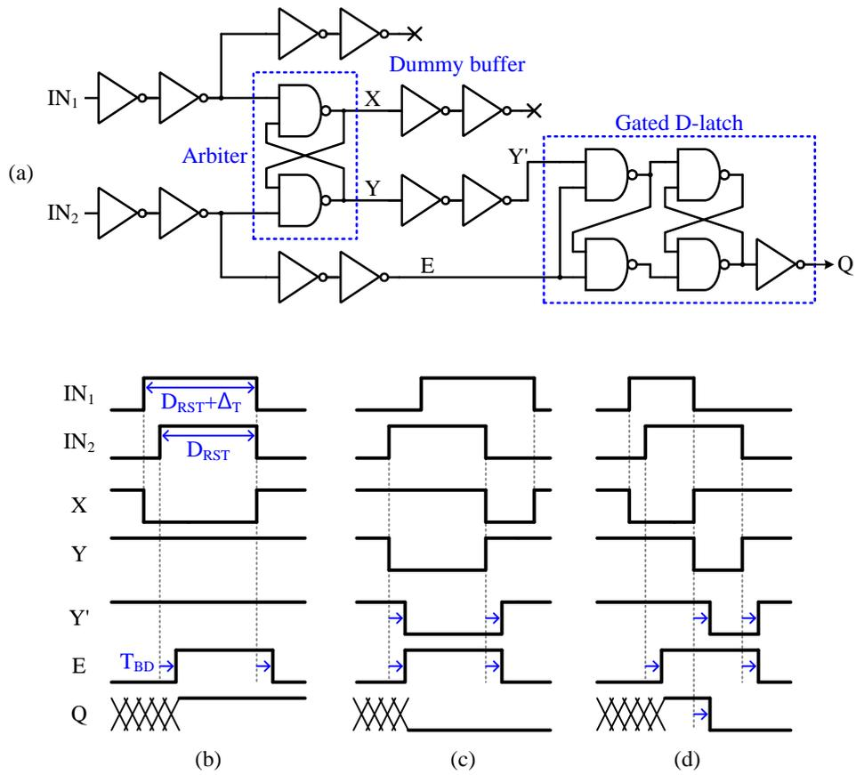
Figure 2.14: (a) Schematics of proposed arbiter-based PDC circuit, timing diagram with the case of (b)  $IN_1$  first, (c)  $IN_2$  first, (d) error
