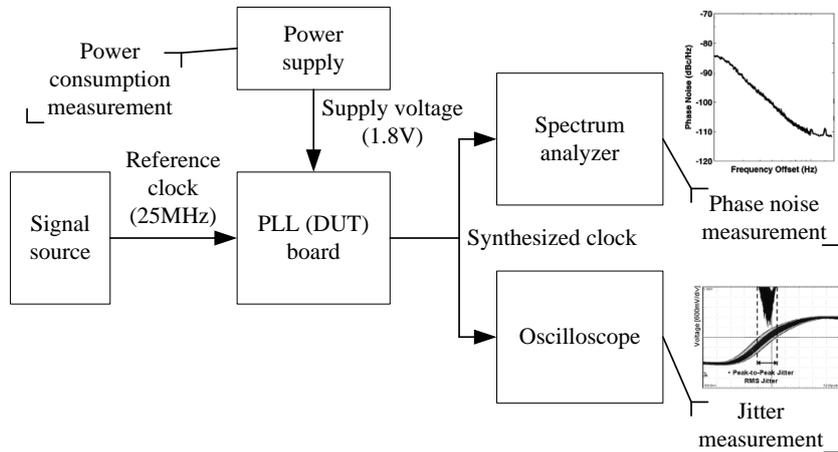
Figure 3.3: PLL Measurement setup
