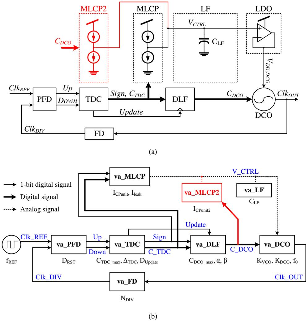
Figure 4.1: (a) Block-diagram of modified PLL including an AFC compensator, (b) simulation test-bench
