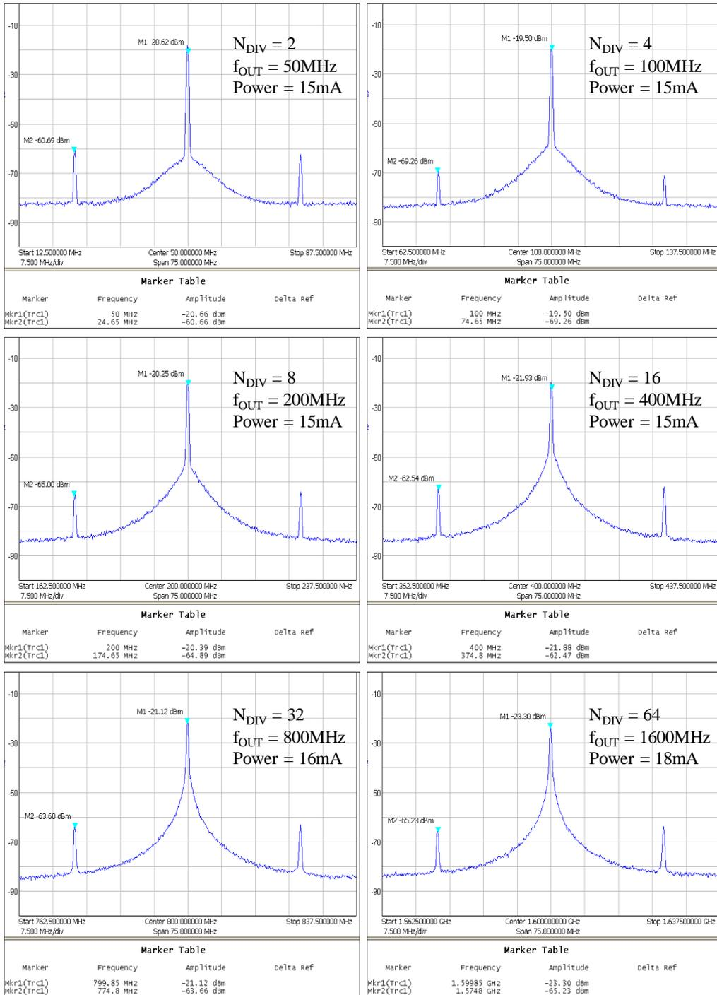
Figure 3.6: PSD results of output clock with  $N_{DIV}$  variations from 2 to 64
