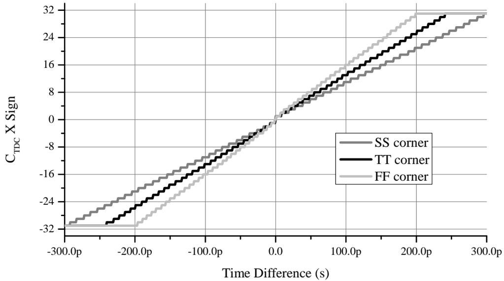
Figure 2.18: Simulated transfer function of PFD-TDC using our PDC
