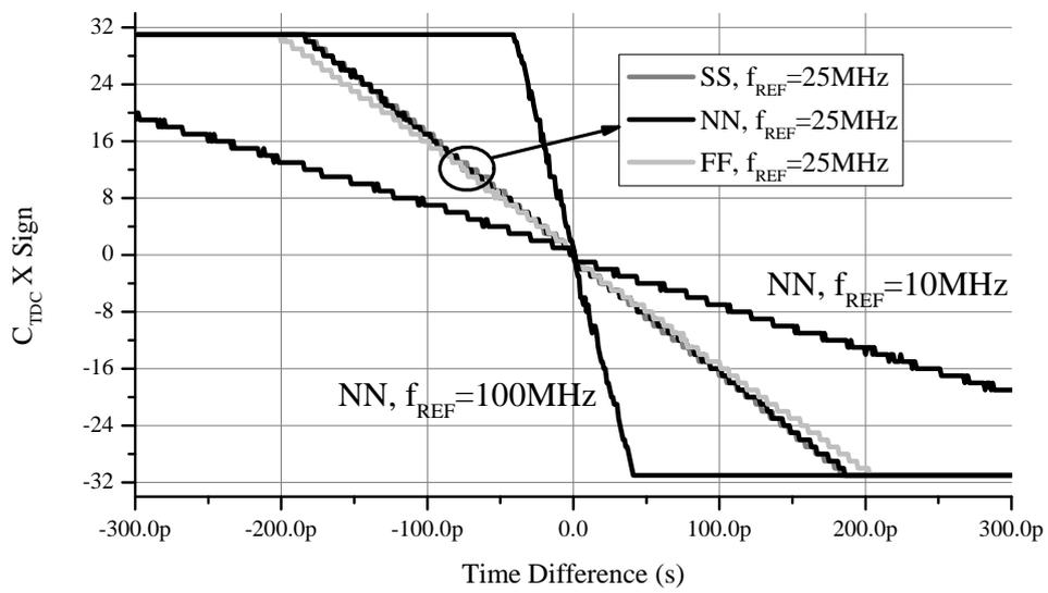
Figure 4.17: TDC curve simulation results with  $f_{REF}$  variations and process corner variations
