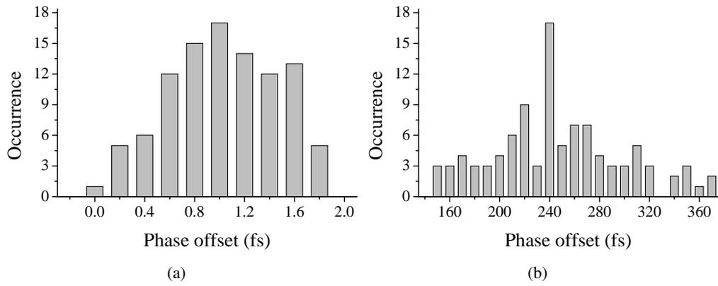
Figure 2.15: Monte-Carlo phase offset simulation results of (a) proposed arbiter-based PDC, (b) time-amp-based PDC
