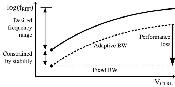
Figure 4.6: Adaptive bandwidth versus fixed bandwidth in case of a wide frequency range
