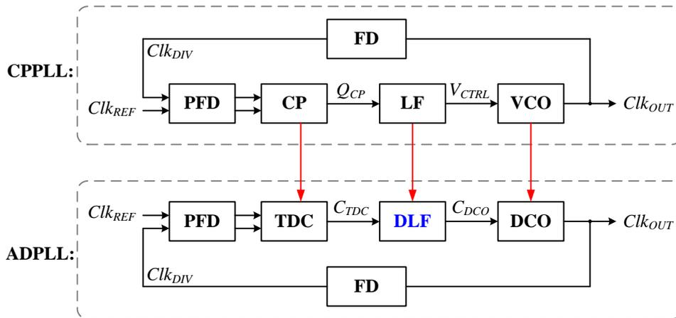
Figure 1.4: Block-diagram comparison between CPPLLs and ADPLLs
