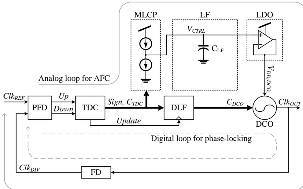
Figure 2.2: Block-diagram of proposed PLL
