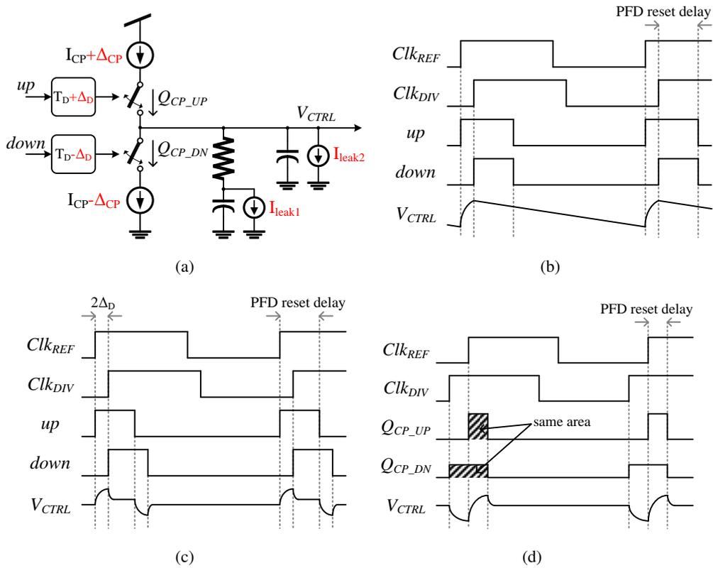
Figure 1.3: (a) CPPLL non-ideality model, effect of (b) gate-tunneling leakage current, (c) timing mismatch, (d) current mismatch
