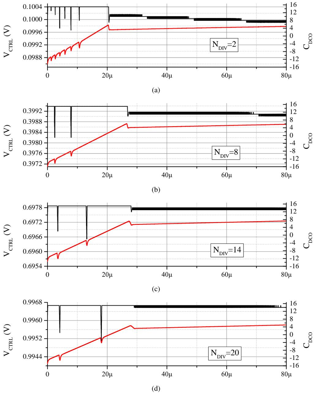
Figure 4.11: Behavioral simulation results of secondly modified PLL with  $N_{DIV}$  variations
