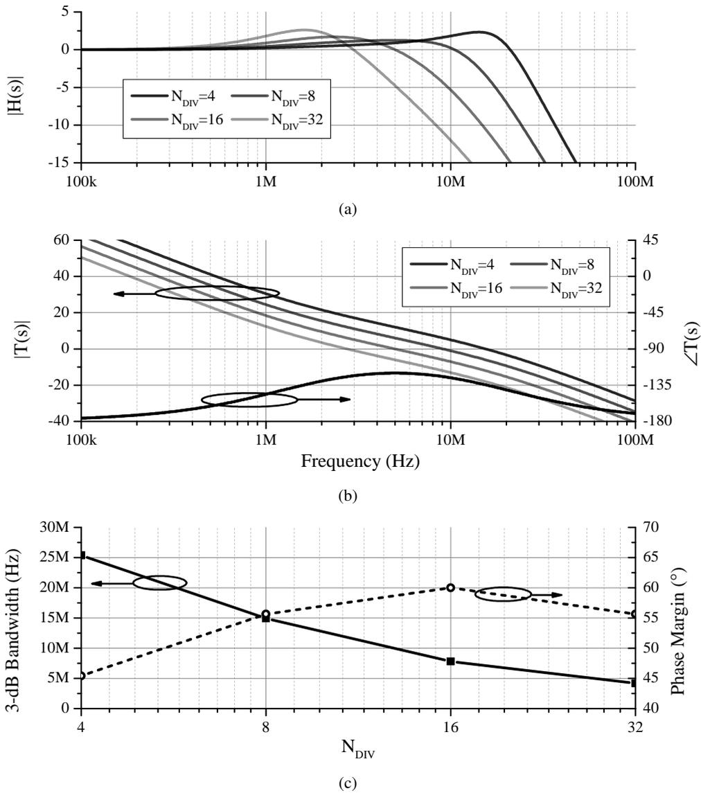
Figure 2.6: Small-signal model simulation results of conventional CPPLL using fixed loop filter with  $N_{DIV}$  variations, (a) closed-loop magnitude response, (b) open-loop magnitude and phase responses, (c) 3-dB bandwidth and phase margin variations
