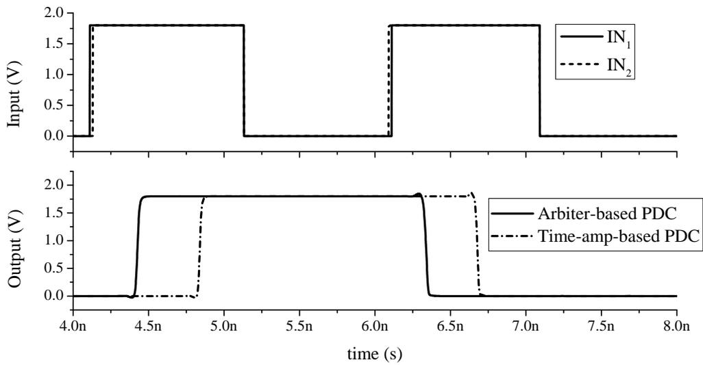
Figure 2.16: Input-to-Q delay simulation results
