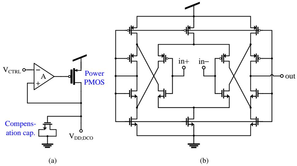
Figure 2.21: Schematics of (a) LDO, (b) OP-Amp
