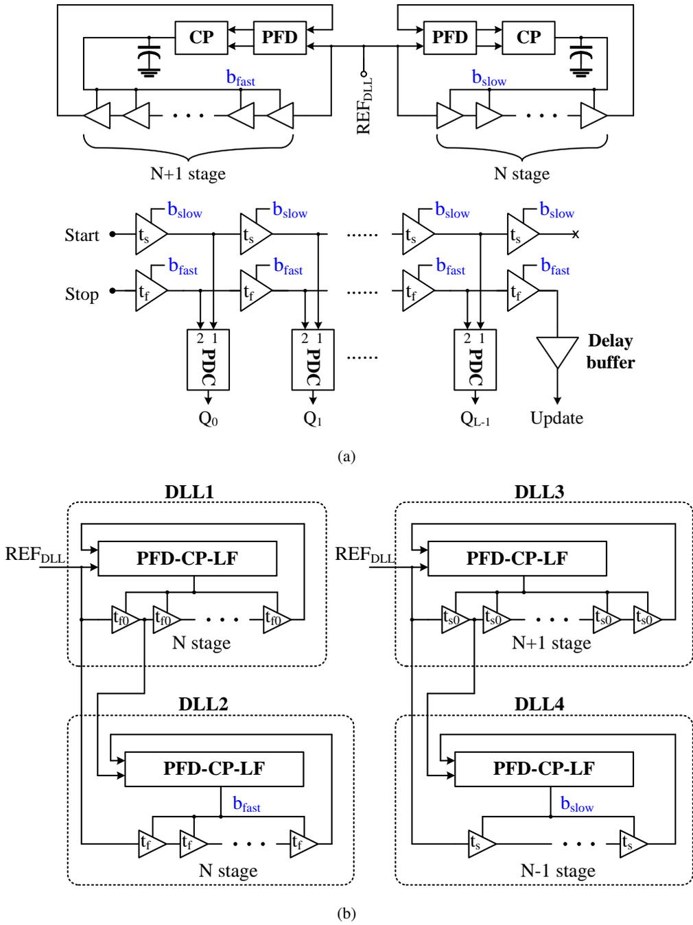
Figure 4.13: Schematics of (a) conventional dual-DLL, (b) proposed quadruple-DLL for  $\Delta T_{DC}$  calibration
