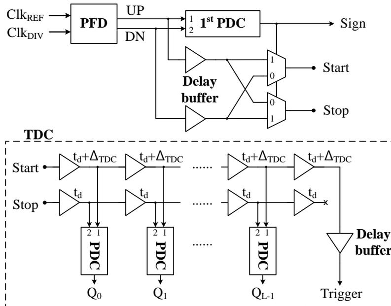
Figure 2.13: Designed combination of PFD and TDC which can avoid offset and dead-zone problems
