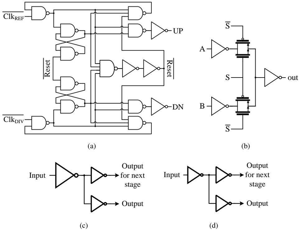
Figure 2.17: Schematics of (a) PFD, (b) MUX, (c) delay cell for fast path, (d) delay cell for slow path in VDL TDC
