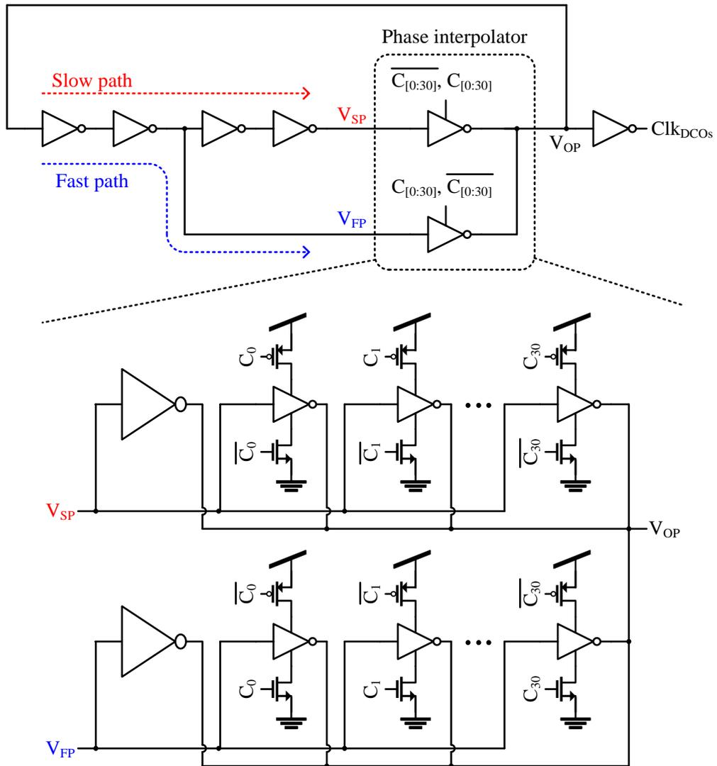
Figure 2.10: Schematics of proposed DCO - oscillator part
