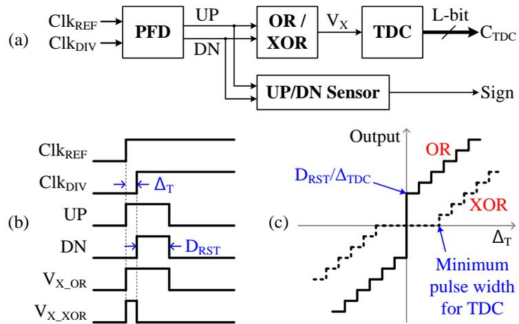
Figure 2.12: (a) Conventional combination of PFD and TDC, (b) timing diagram, (c) potential offset or dead-zone problem
