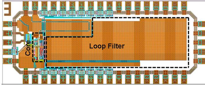
Figure 1.2: Conventional CPPLL layout example
