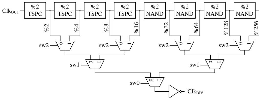
Figure 2.22: Schematics of programmable frequency divider
