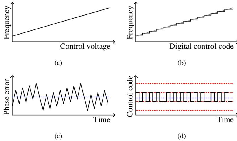
Figure 1.6: Examples of (a) VCO frequency curve, (b) DCO frequency curve, (c) AD-PLL phase error transitions and (d) DCO control code transitions in locked-state
