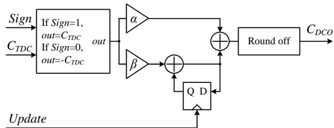
Figure 2.4: Block-diagram showing the DLF operation and linearized model
