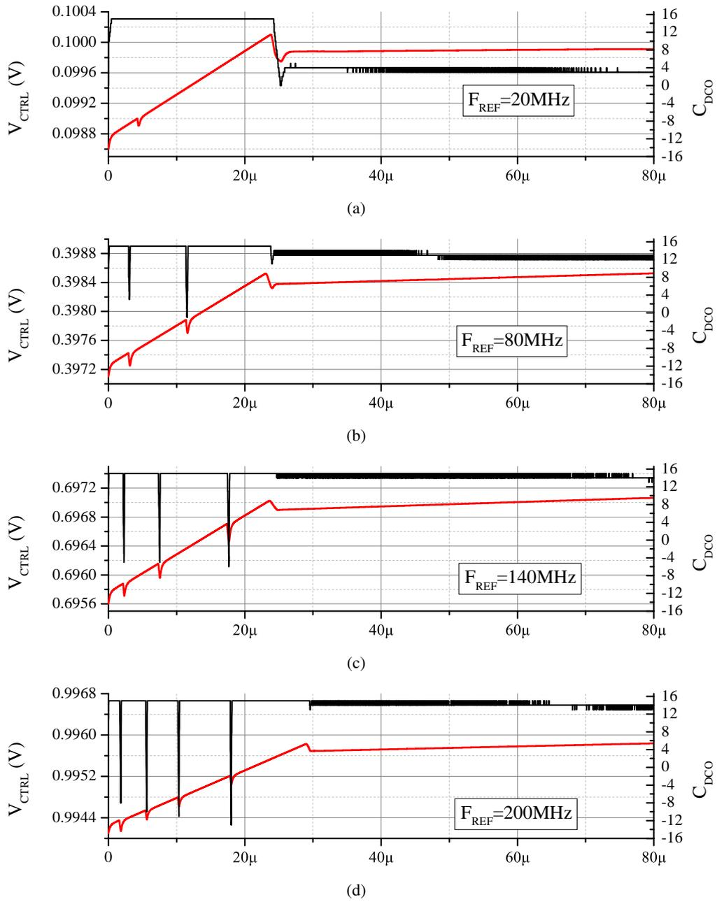
Figure 4.12: Behavioral simulation results of secondly modified PLL with  $f_{REF}$  variations
