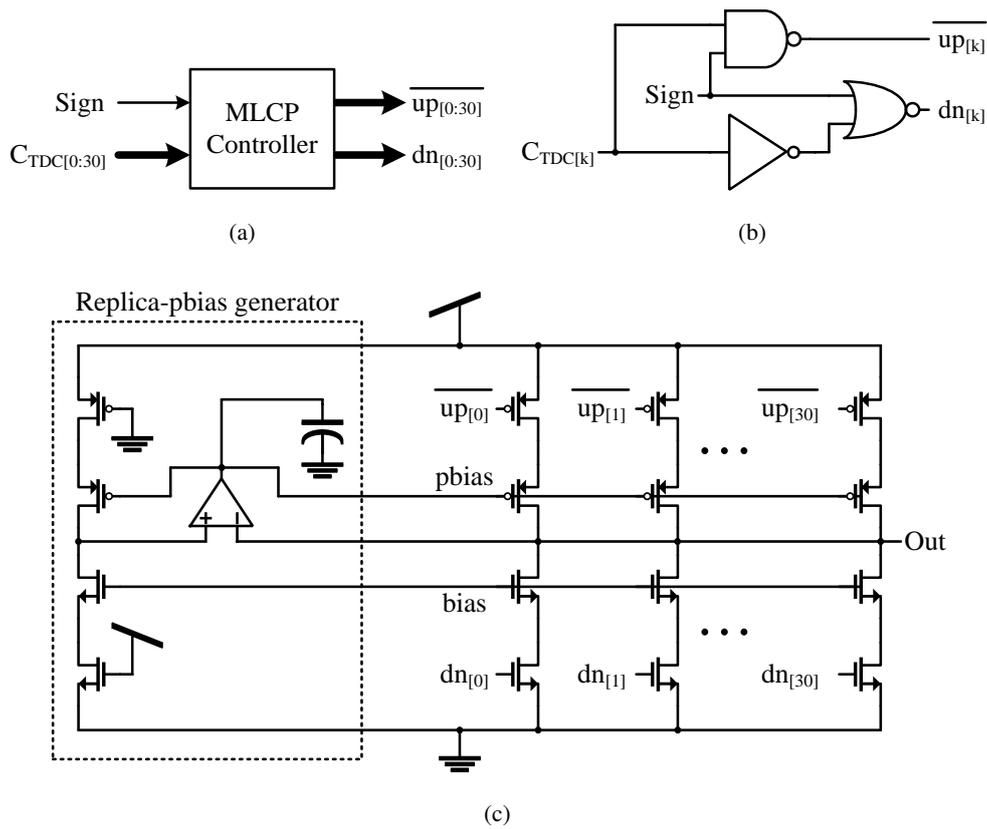
Figure 2.20: (a) MLCP controller, schematics of (b) MLCP controller cell, (c) MLCP core
