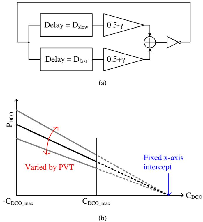
Figure 2.9: (a) Conceptual block-diagram of proposed DCO, (b) oscillation period curve examples with PVT variations
