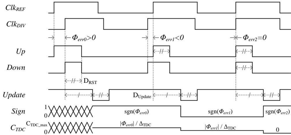
Figure 2.3: Timing diagram showing the operation of PFD and TDC
