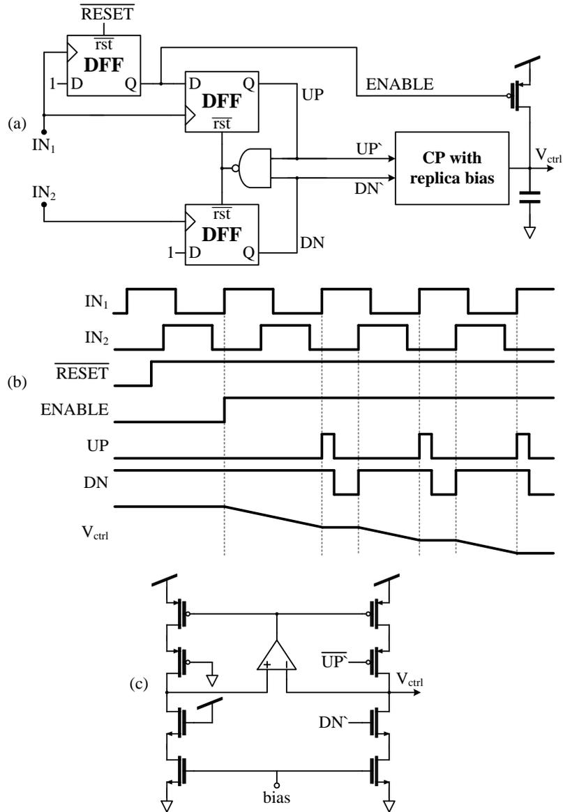
Figure 4.14: (a) Schematics of PFD and CP for DLL to avoid harmonic-lock problem, (b) timing diagram, (c) pulse reshape circuit, (d) CP circuit
