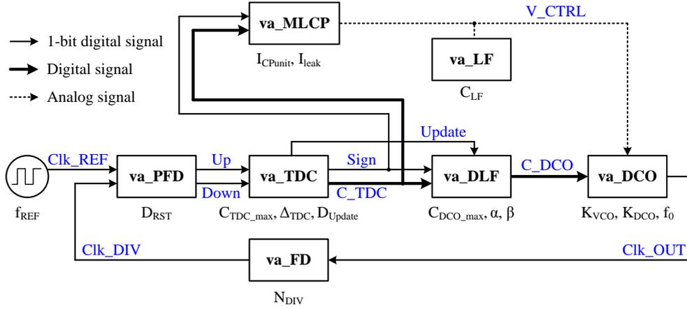
Figure 3.7: Behavioral simulation test-bench for problem analysis
