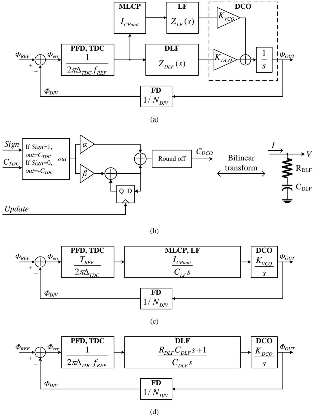
Figure 2.5: (a) Small-signal model of proposed dual-loop PLL, (b) linearized DLF model, (c) AFC loop only, (d) digital loop only
