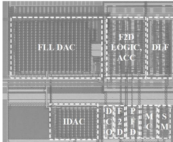
Figure 2.1: Layout example of a conventional wide-range ADPLL [9]. Total chip area is  $0.27\text{mm}^2$ , where DCO and DACs occupy an area of more than half.
