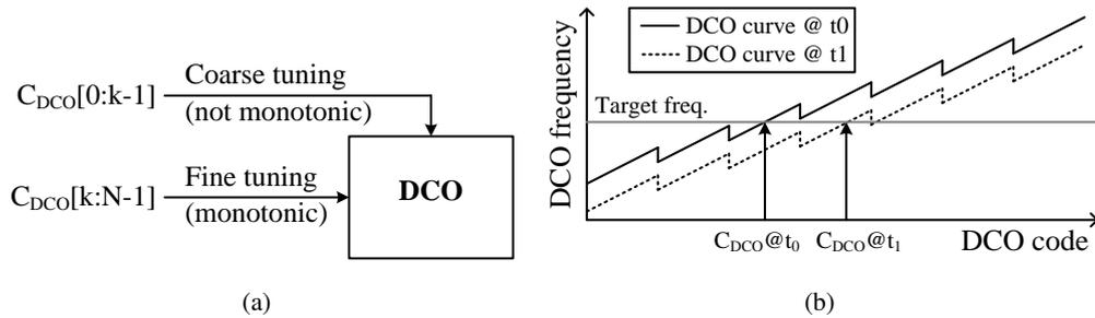
Figure 1.7: (a) Multi-band DCO, (b) example of DCO frequency curve variation depending on the time
