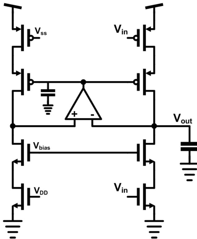
Figure 2-11. Schematic of charge-pump with p-n current matching
