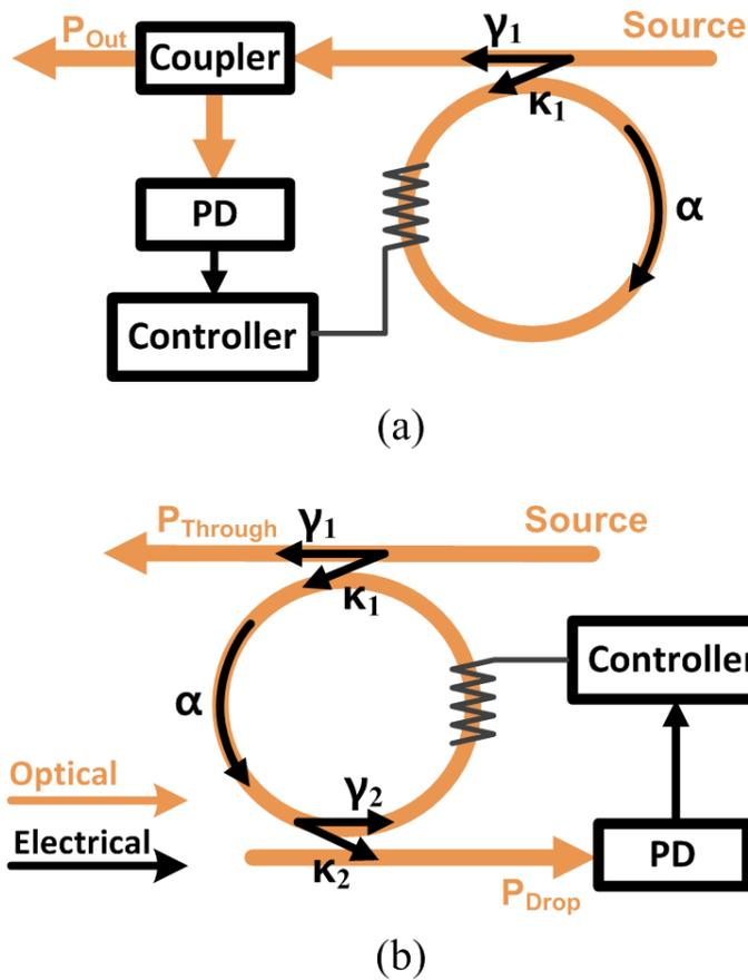
Figure 1-11. Conceptual block diagram of the Si MRM wavelength ( $\lambda$ ) stabilization circuit (a) without or (b) with a drop port
