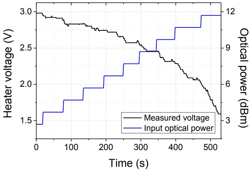
Figure 4-20. Input optical power variations to Si MRM and measured heater voltages controlled by the  $\lambda$ -stabilization circuit
