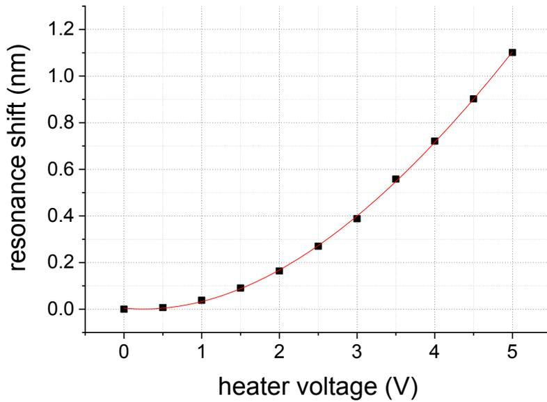
Figure 4-4. Heater I-V curve, resistance, and resonance wavelength change according to its voltages
