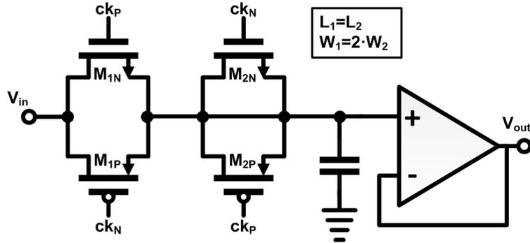
Figure 2-8. Schematic of CMOS T/H circuit with charge-offset cancellation
