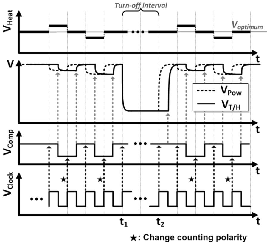
Figure 4-8. Timing diagram of low-power continuous-time calibration step (Second step)
