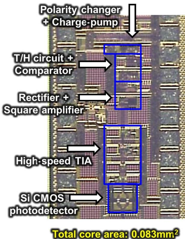
Figure 2-13. Microphotograph of bias controller IC chip
