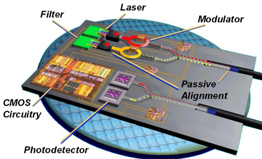
Figure 1-2. Conceptual structure of Si photonics [11]
