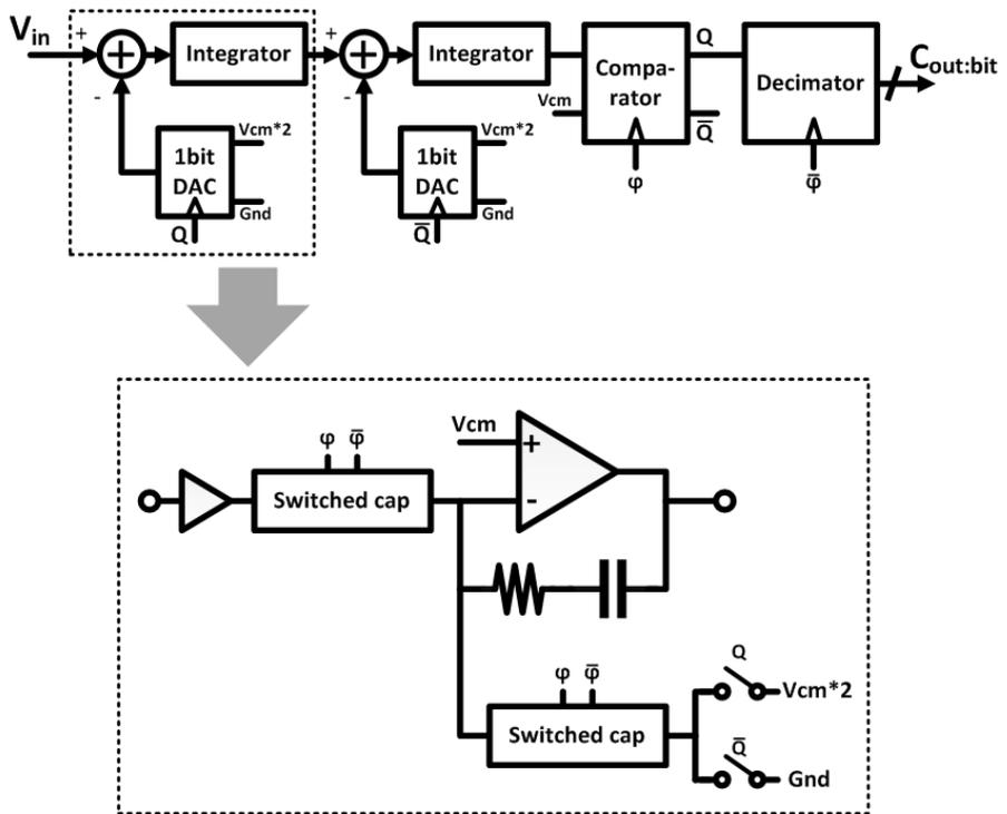
Figure 3-7. Schematic of analog-to-digital converter (ADC) based on second-order delta-sigma ( $\Sigma$ - $\Delta$ ) modulator
