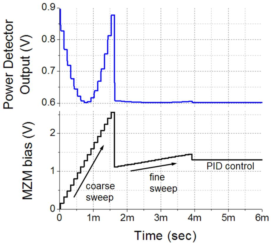
Figure 3-10. Simulated MZM bias voltage and power detector's output at initial bias scan step (First step)
