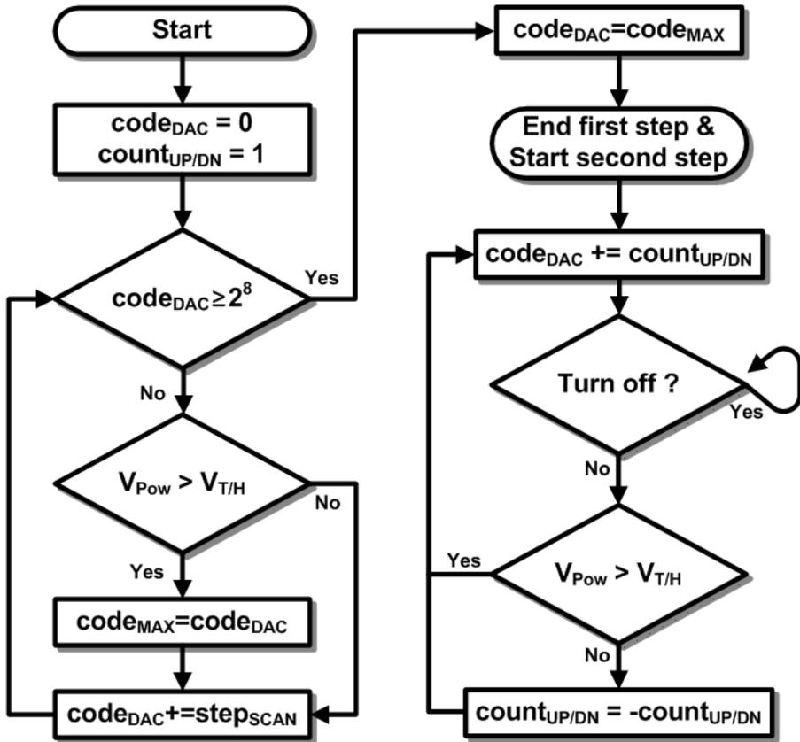
Figure 4-6. Algorithm flowchart of two-step approach based on low-power OMA monitoring
