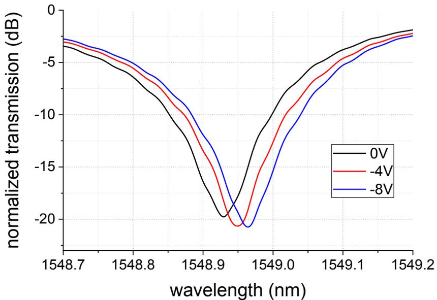
Figure 4-3. Si MRM transmission spectra according to three different DC biases
