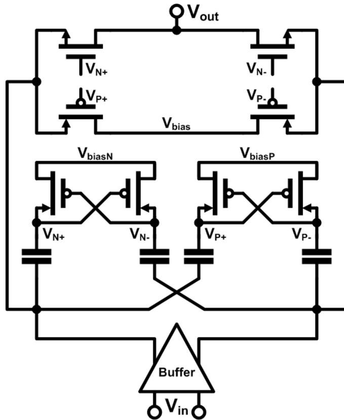
Figure 2-5. Schematic of driven-gate CMOS high-speed rectifier
