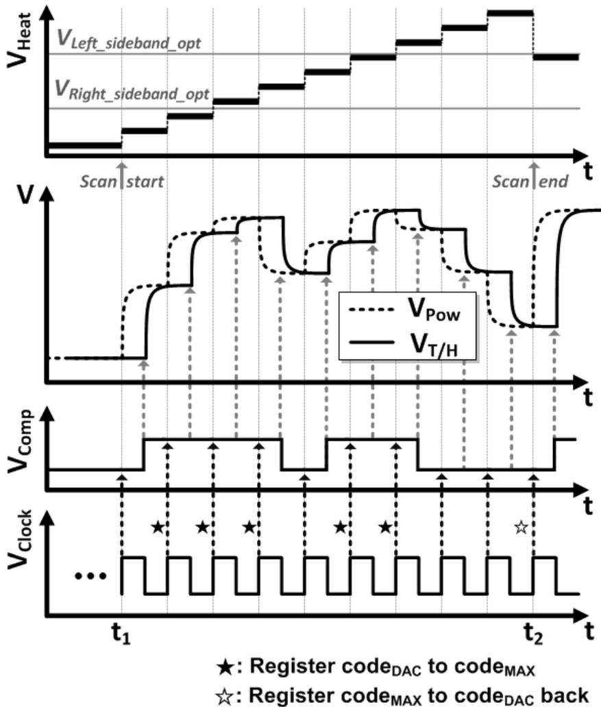
Figure 4-7. Timing diagram of initial bias scan step (First step)
