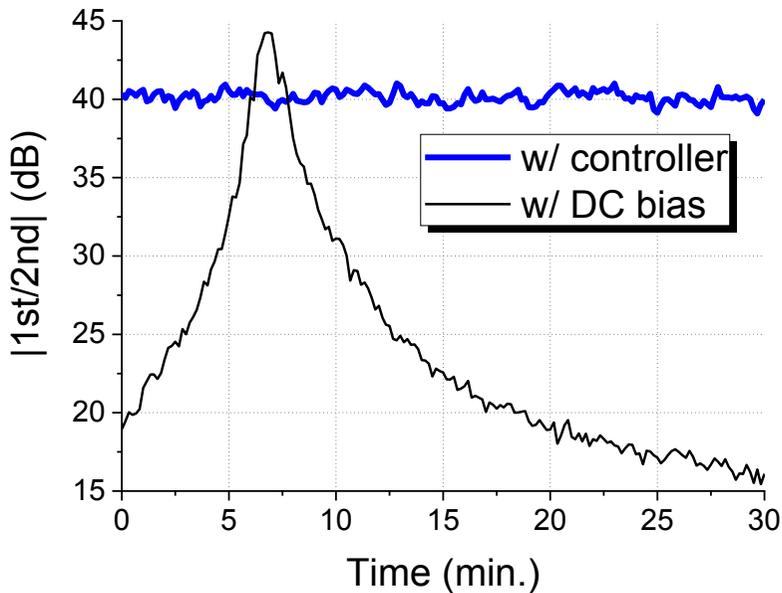
Figure 2-16. Ratio of first and 2nd-harmonic components for 1.5-GHz modulation of MZM with and without bias controller
