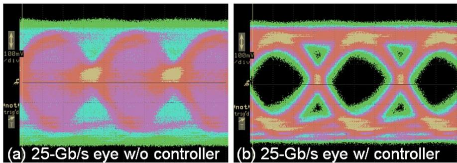
Figure 3-15. Measured eye diagrams of 25-Gb/s PRBS7 accumulated for 6 minutes (a) without and (b) with the bias controller while bias noises are supplied as shown in Figure 3-13
