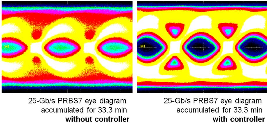
Figure 4-19. Measured eye diagrams of 25-Gb/s PRBS7 accumulated for 33.3 min (a) without and (b) with the  $\lambda$ -stabilization circuit while external temperature variations are supplied as shown in figure 4-20
