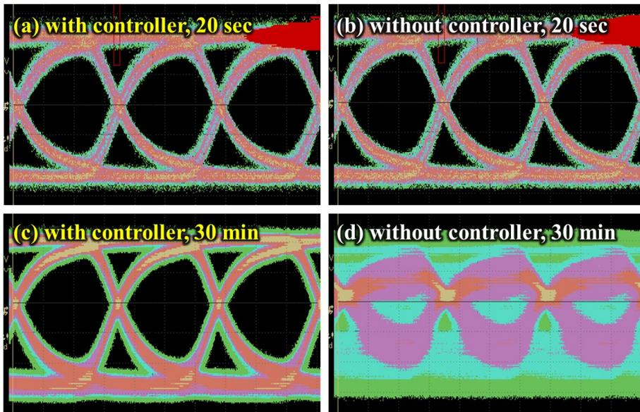
Figure 2-17. Accumulated eye diagram of 3-Gb/s data modulated with LiNbO<sub>3</sub> MZM with or without bias controller (a), (b) for initial 20 seconds and (c), (d) for 30 minutes
