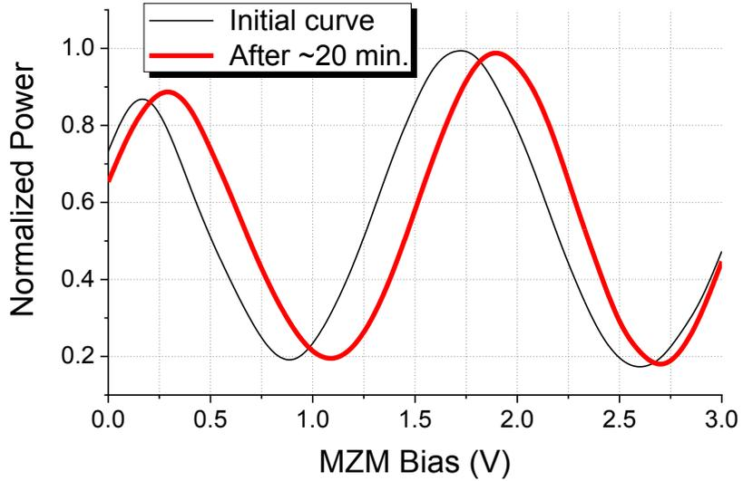
Figure 1-5. Normalized optical power transfer curve of LiNbO3 MZM
