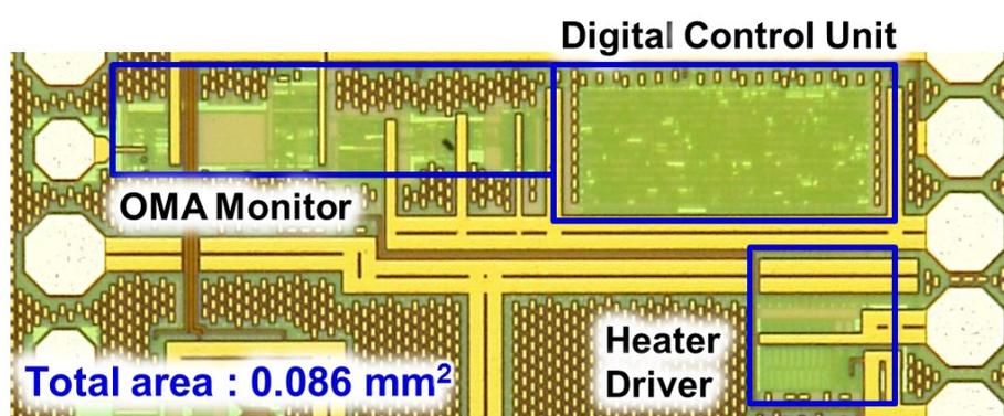
Figure 4-14. Photograph of  $\lambda$ -stabilization IC chip
