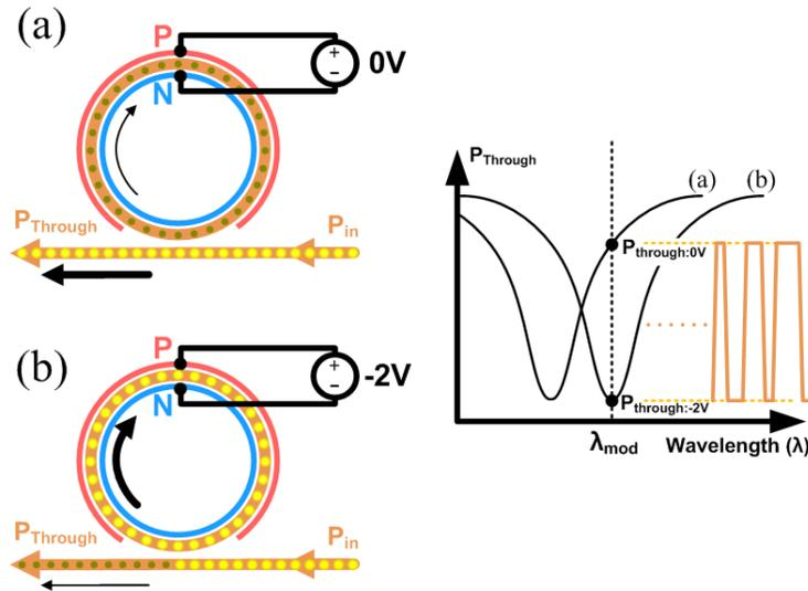
Figure 1-7. Conceptual optical modulation diagram with MRM transmission spectra
