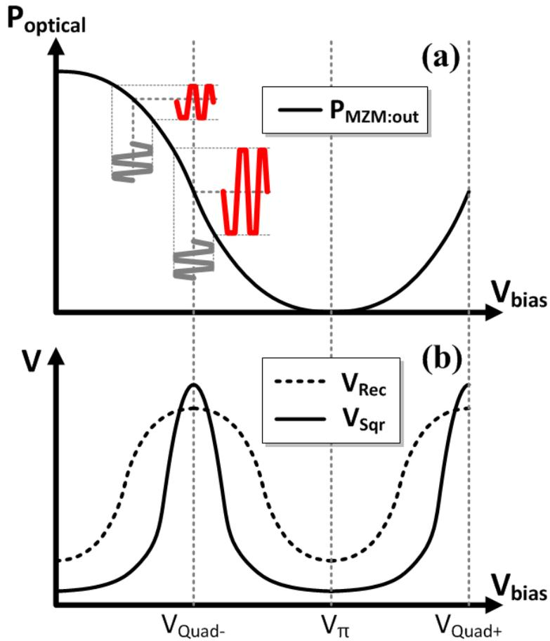
Figure 2-2. (a) MZM DC bias transfer curve with (b) rectifier output ( $V_{\text{Rec}}$ ) and square amplifier output ( $V_{\text{Sqr}}$ )
