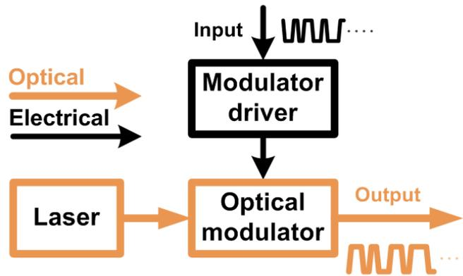
Figure 1-3. Conceptual block diagram of optical transmitter
