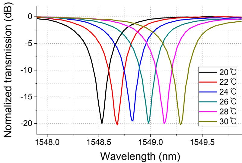
Figure 1-8. Si MRM transmission spectra according to six different external temperatures
