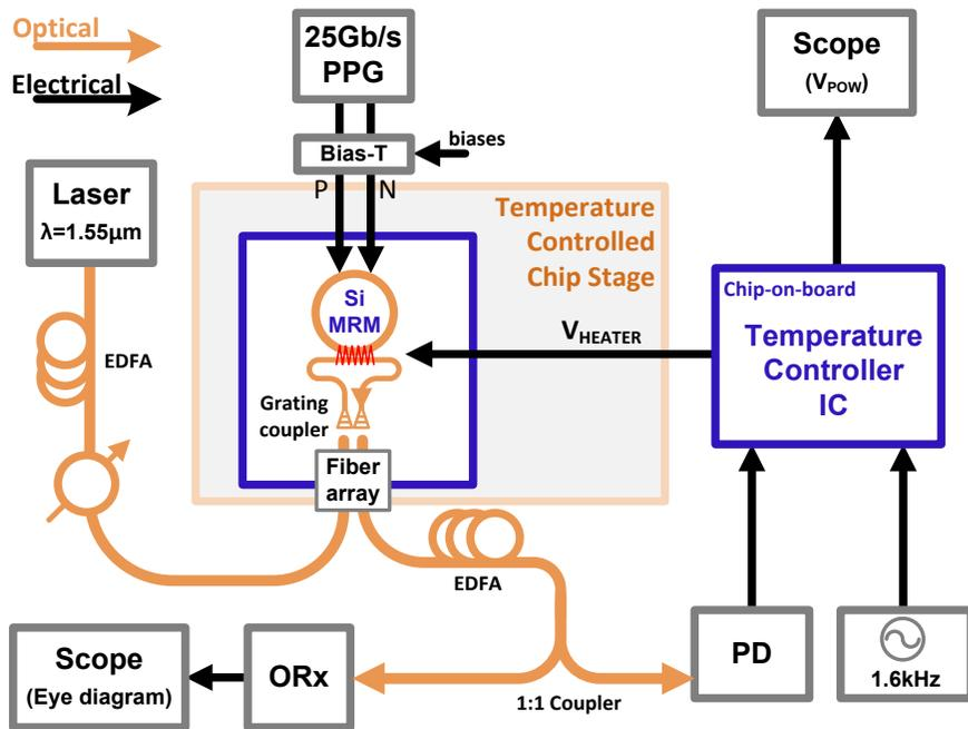
Figure 4-15. Measurement setup for demonstration of  $\lambda$ -stabilization circuit for Si MRM
