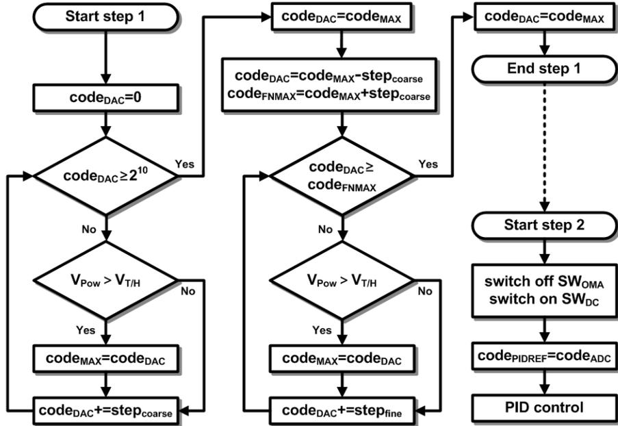
Figure 3-2. Algorithm flowchart of MZM bias control based on OMA and average power monitoring
