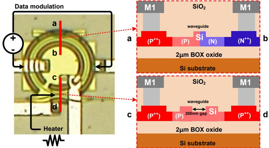
Figure 4-2. Physical structure and cross-sections of Si MRM
