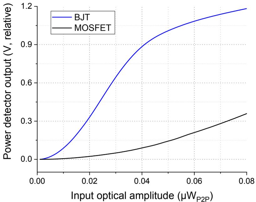
Figure 4-9. Simulation comparison between CMOS and BJT according to input pair on power detector
