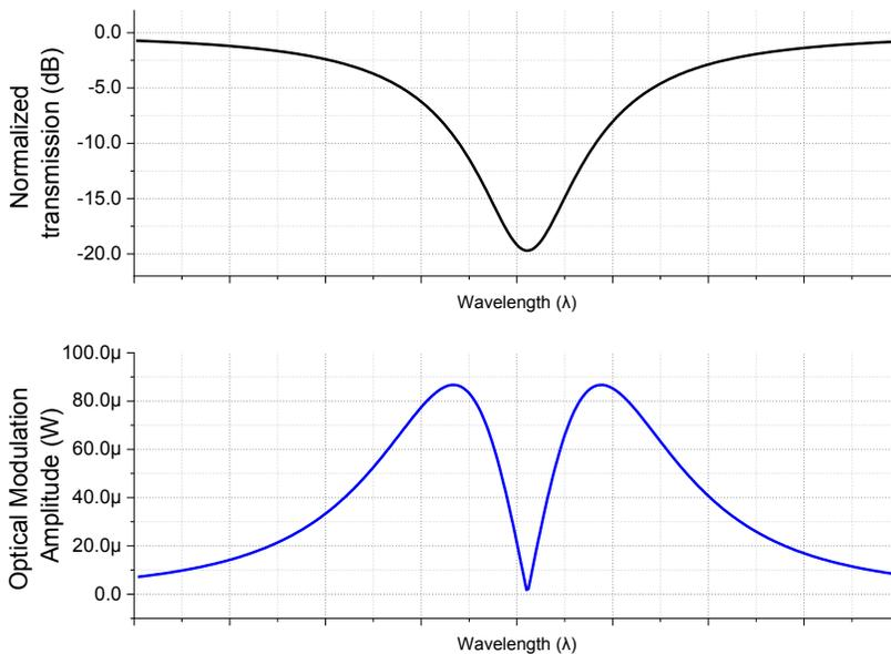
Figure 4-1. Si MRM spectra of normalized DC transmission with 0-V and OMA transmissions with  $\pm 4$ -V modulation
