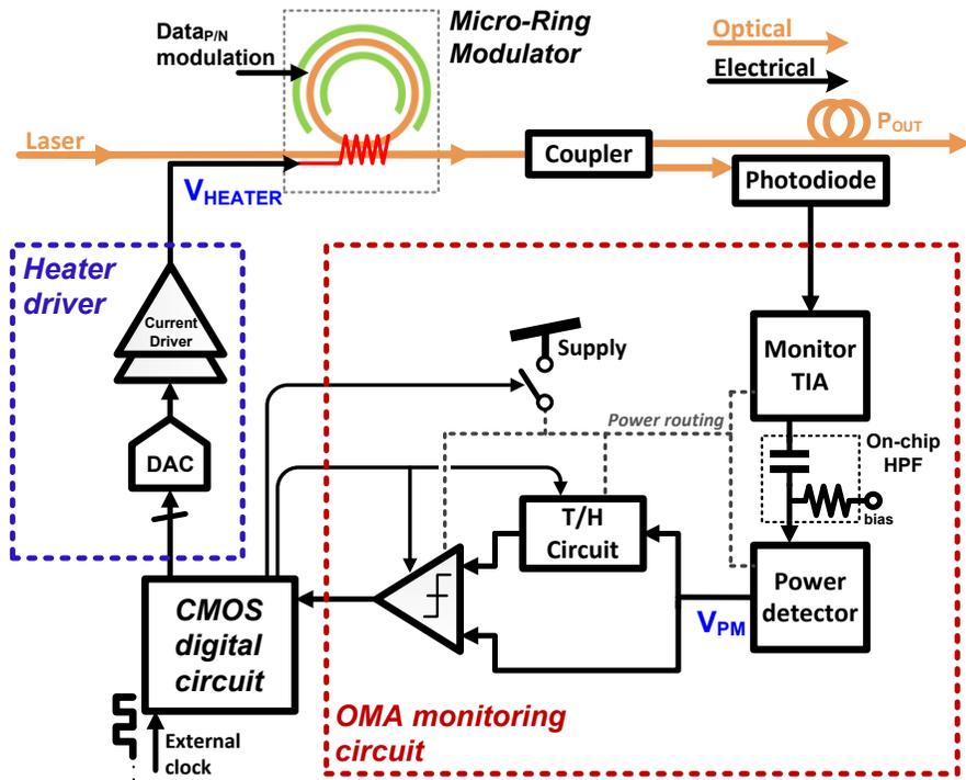
Figure 4-5. Block diagram of Si MRM wavelength ( $\lambda$ ) stabilization circuit based on low-power OMA monitoring
