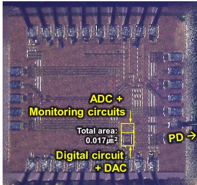
Figure 3-11. Photograph of bias controller IC chip
