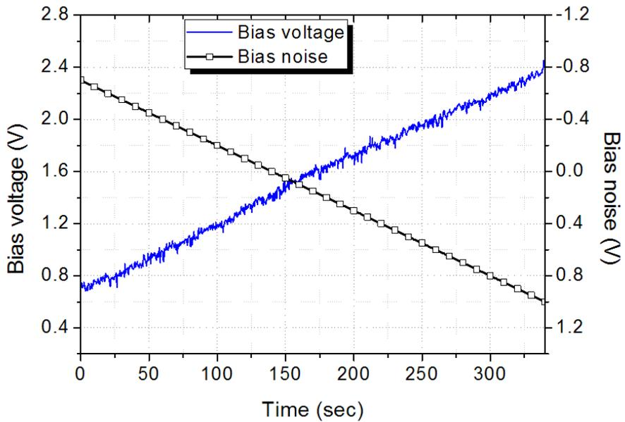
Figure 3-14. Bias noise transient into MZM RF port and measured MZM bias voltages determined by the bias controller
