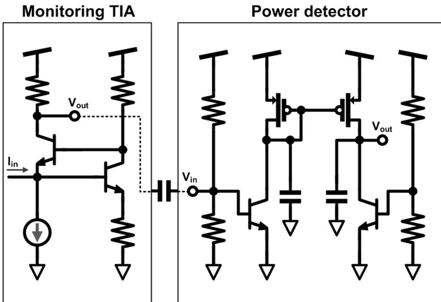
Figure 4-10. Schematic of regulated-cascode TIA and power detector based on BJT
