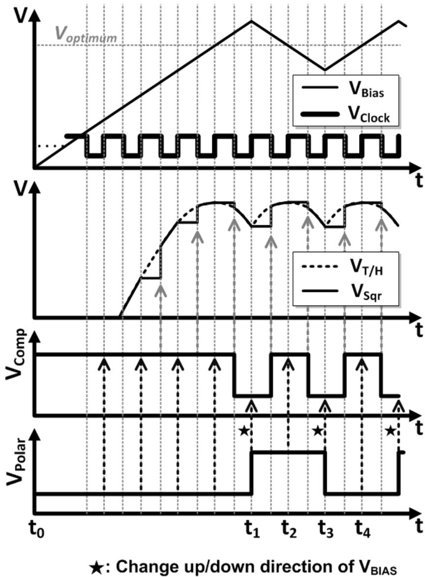
Figure 2-3. Timing diagram of bias control process
