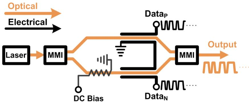
Figure 1-4. Basic structure of Mach-Zehnder modulator (MZM)
