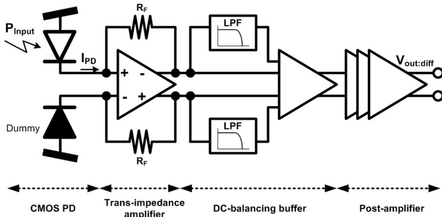
Figure 2-4. Schematic of shunt-shunt feedback TIA
