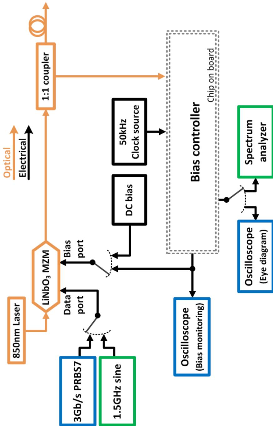
Figure 2-14. Measurement setup for demonstration of MZM bias controller based on OMA monitoring
