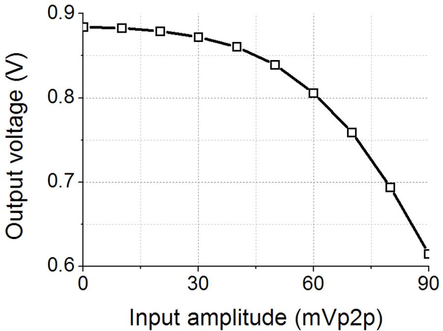
Figure 3-6. Post-layout simulation results of CMOS power detector
