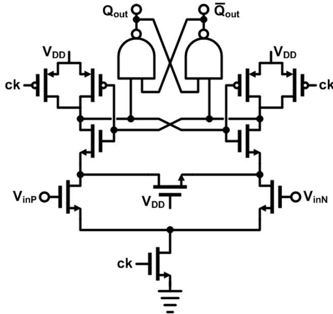
Figure 2-9. Schematic of sense-amplifier-based D flip-flop
