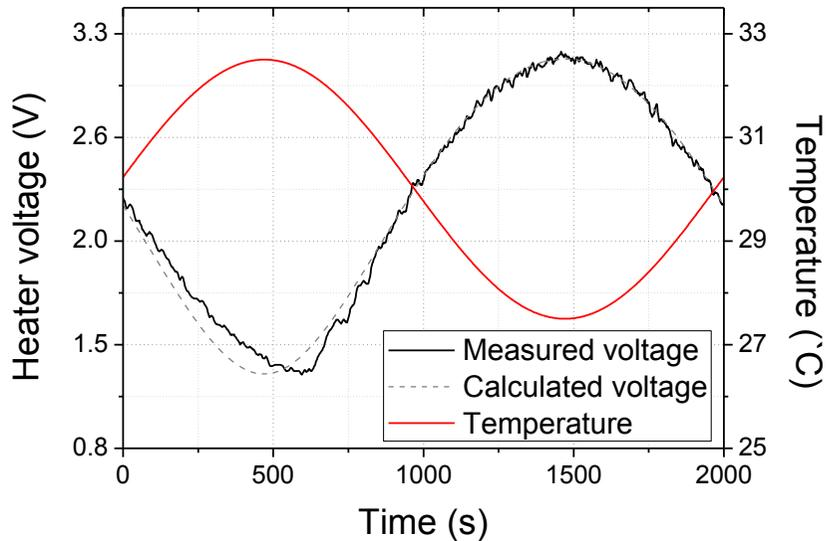
Figure 4-18. External temperature variations to Si MRM and measured heater voltages controlled by the  $\lambda$ -stabilization circuit
