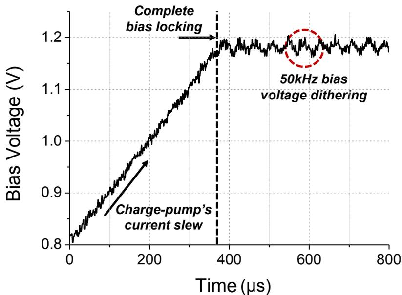
Figure 2-15. Initial transient response of MZM bias voltage
