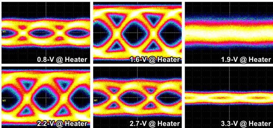
Figure 4-17. Measured eye diagrams according to six different heater voltages
