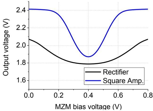
Figure 2-7. Simulation results of rectifier and square amplifier outputs according to MZM DC bias
