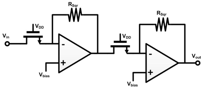
Figure 2-6. Schematic of CMOS square amplifier
