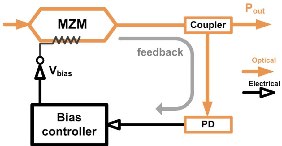
Figure 1-10. Conceptual block diagram of the MZM bias controller
