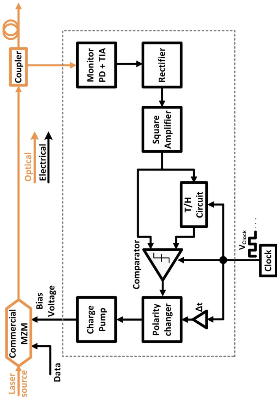
Figure 2-1. Block diagram of MZM bias controller based on OMA monitoring
