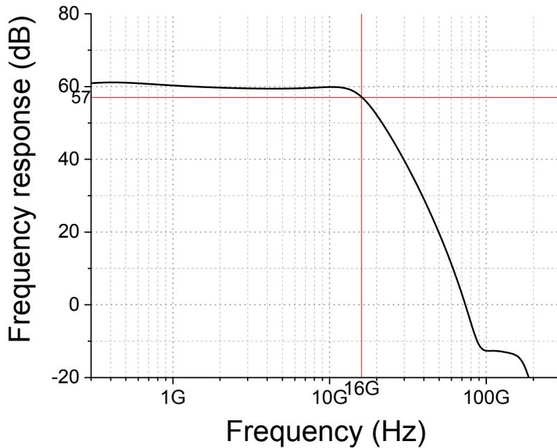
Figure 4-11. Post-layout frequency response simulation result of TIA
