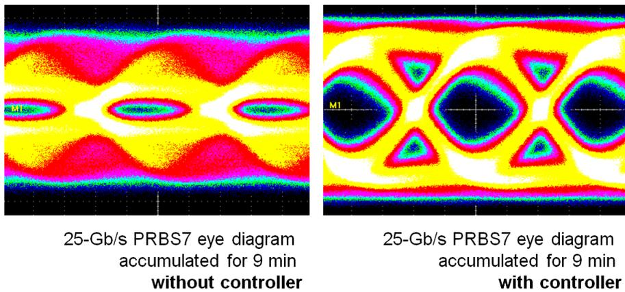
Figure 4-21. Measured eye diagrams of 25-Gb/s PRBS7 accumulated for 9 min (a) without and (b) with the  $\lambda$ -stabilization circuit while input optical power variations are supplied as shown in figure 4-22
