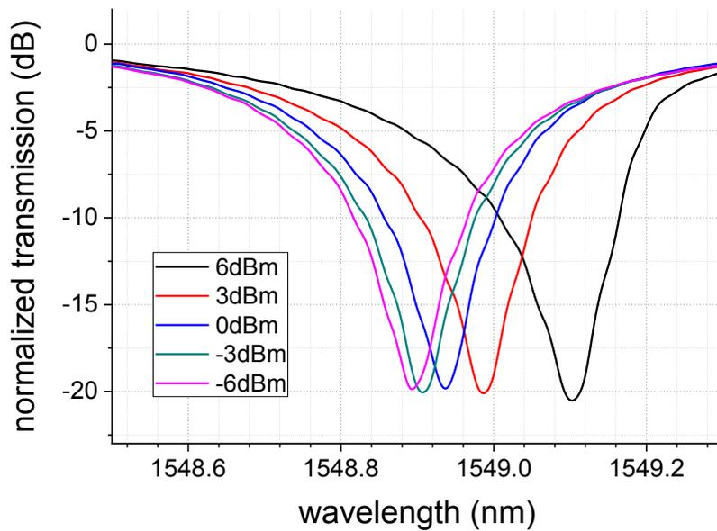
Figure 1-9. Si MRM transmission spectra according to five different input optical powers
