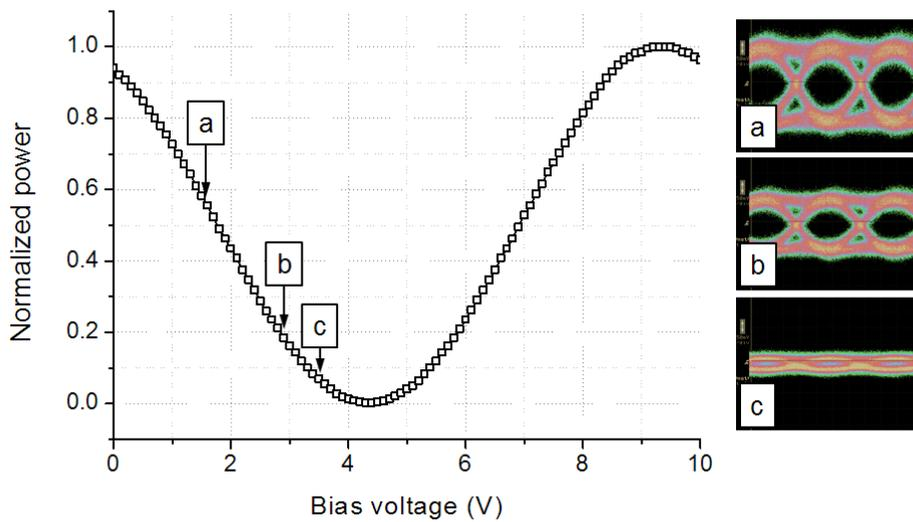
Figure 3-13. DC characteristic curves of 1550-nm MZM used in measurement and modulated eye diagrams according to three different bias voltages
