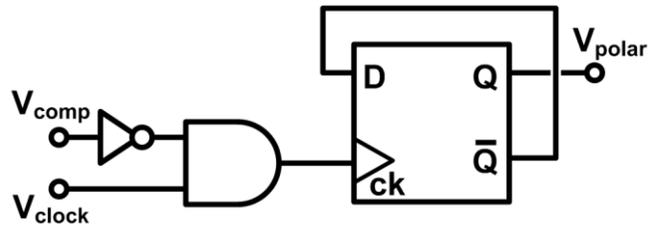
Figure 2-10. Schematic of polarity changer
