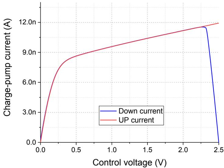
Figure 2-12. Simulation results of charge-pump currents according to output voltage
