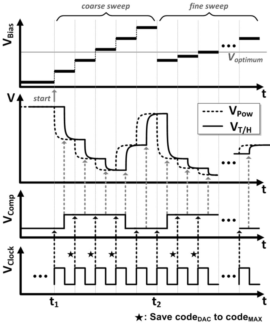
Figure 3-3. Timing diagram of initial bias scan step (First step)
