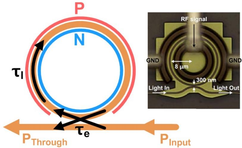
Figure 1-6. Basic structure of Si micro-ring modulator
