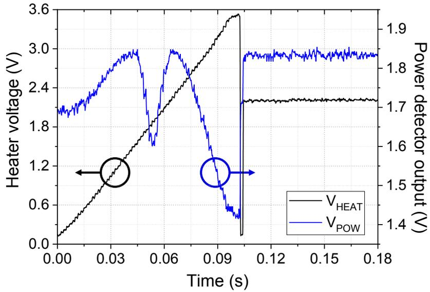
Figure 4-16. Measured transient response of power detector's output according to heater voltage at first initial scan step
