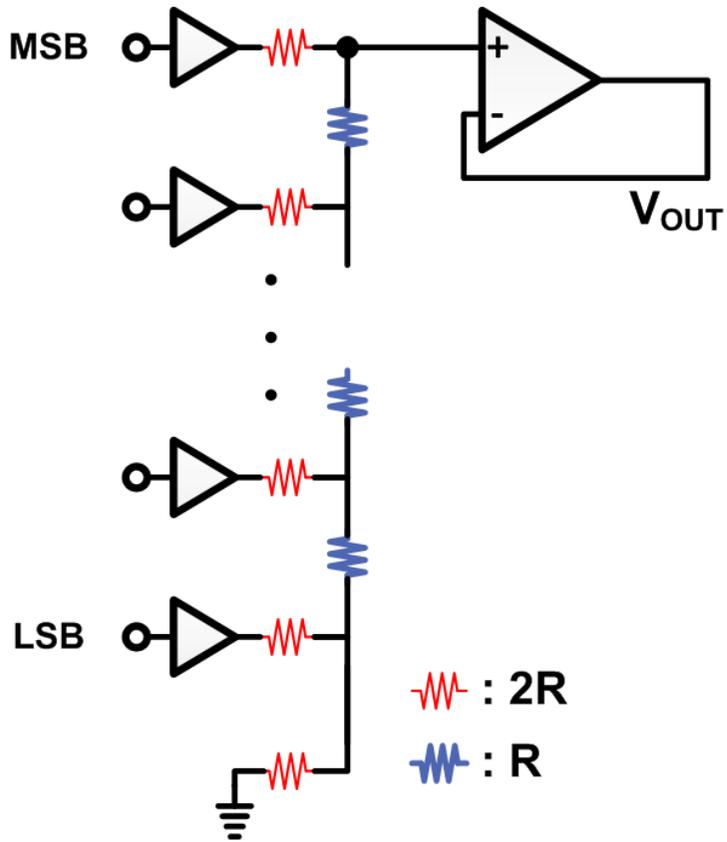
Figure 3-8. Schematic of digital-to-analog converter (DAC) based on R-2R ladder structure
