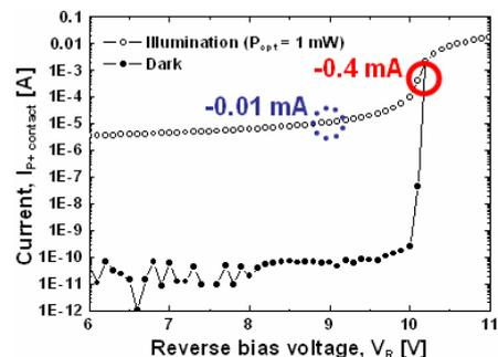
Fig. 2. I-V characteristics of the CMOS-APD under dark and illumination conditions. The incident optical power is 1mW.
