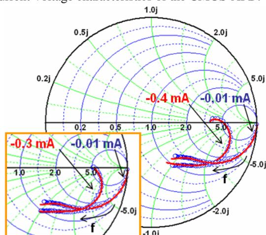
Fig. 3. Comparison of measured and fitted reflection coefficient of p+ port (from 50 MHz to 13.5 GHz). The hollow circles represent measured data and solid lines indicate fitting results.
