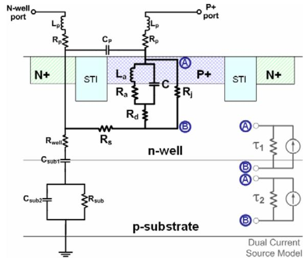
Fig. 1. CMOS-APDs model based on its physical structure.
