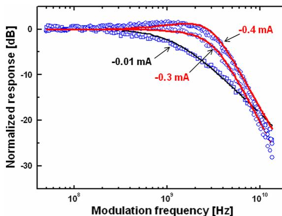
Fig. 4. Comparison of measured and fitted photodetection frequency responses of the CMOS-APD. The symbols represent measured data and solid lines indicate fitting results.
