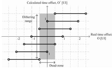
Figure 3: Effect of finite time resolution
