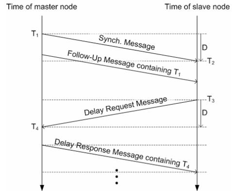
**Figure 1:** One set of message exchange between master and slave nodes to measure time offset and delay
