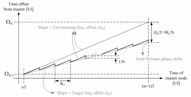
Figure 5: Generation of effective frequency offset using phase adjustment
