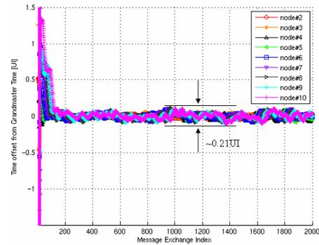
**Figure 8:** Time offsets of serially chained nine nodes from the time of grandmaster. (Filtered TOD value)
