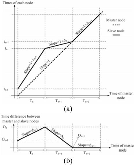
**Figure 2:** Simplified synchronization model with clock rate adjustment: (a) times of each node vs. time of master node (b) time offset between slave and master nodes vs. time of master node.
