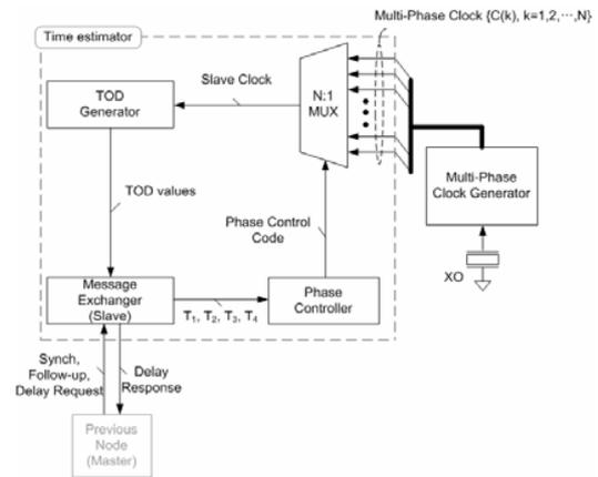
Figure 6: Block diagram of clock synchronization system using phase adjustment
