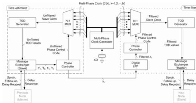
**Figure 7:** Complete block diagram of proposed clock synchronization system
