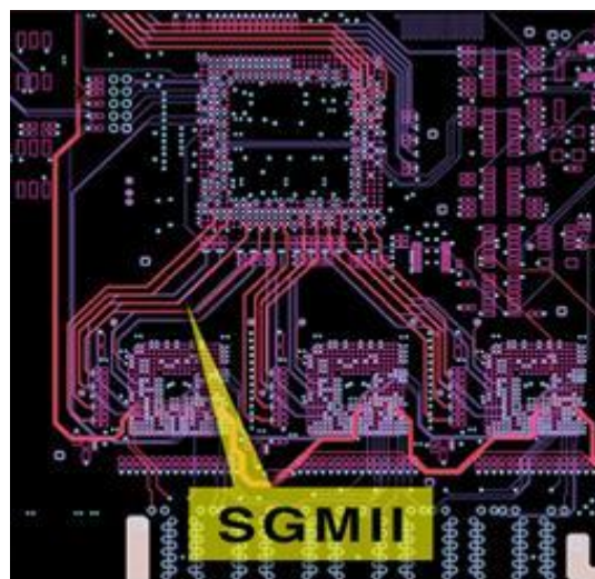
Serial Gigabit Media Independent Interface (SGMII) : Total 8 lines for 1.25 Gb/s
